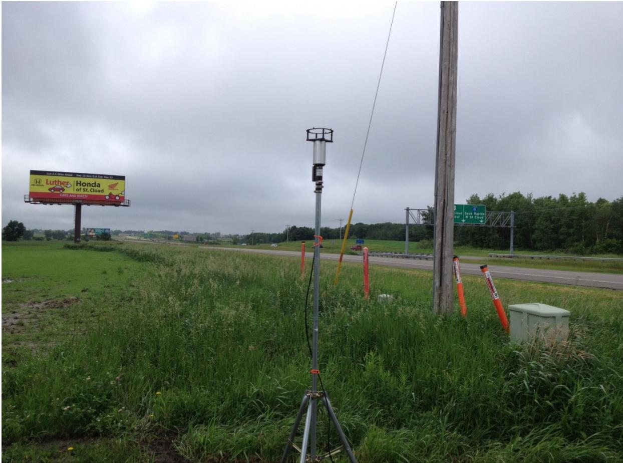
**Figure 4.3 Ultrasonic anemometer near TH 10.**
