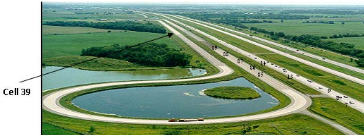
Figure 9.1. MnROAD test facility and cell locations. Cell 85 = pervious concrete on sand, cell 86 = porous asphalt on sand, cell 87 = pervious controls, cell 88 = porous asphalt on clay, cell 89 = pervious concrete on clay, cell 39 = pervious concrete overlay. (Izevbekhai and Akkari 2011).
