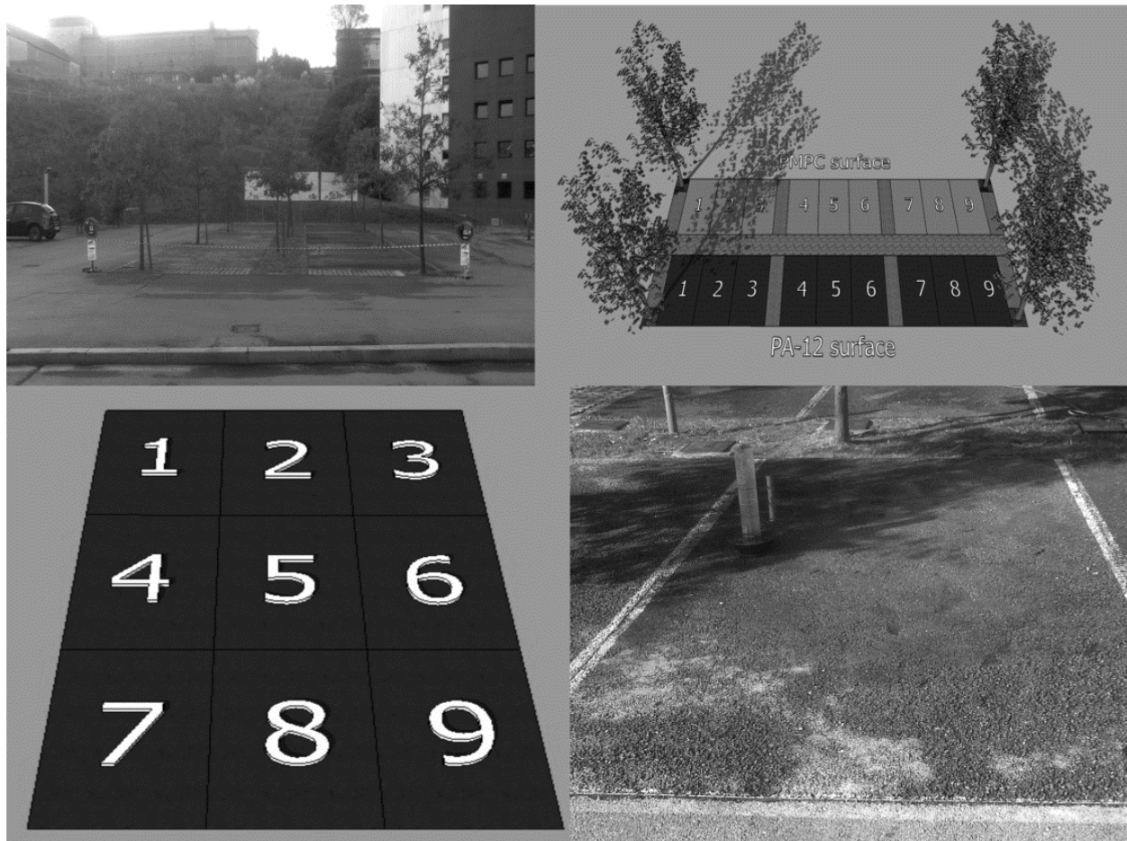
Figure B4-4. (A) Scheme of the eighteen car parking bays analyzed; and (B) measurement zones selected within each car park bay and LCS on-site (Sañudo-Fontaneda et al. 2014).
