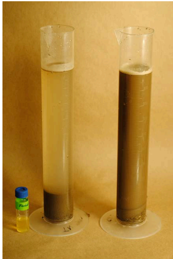
Figure 1: Chitosan flocculent treatment (on left) of Minnesota River silt at ~200g/L. Photo taken 75 seconds after addition of flocculent.
