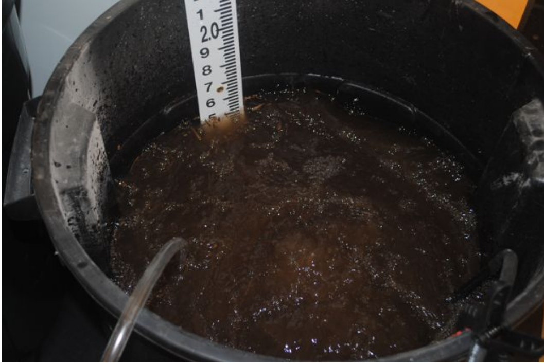
Figure 6. Turbid water stock prepared in a 30 gallon polyethylene container from soil sediment and tap water mixed by injection of air into bottom of fluid column. Staff gage units are feet of depth.
