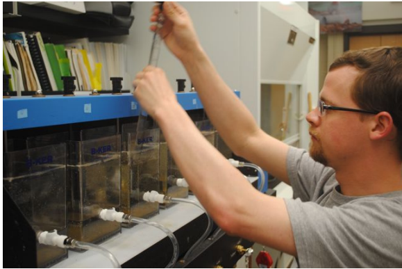
c) Sampling of flocculant-treated water after being allowed to settle.
