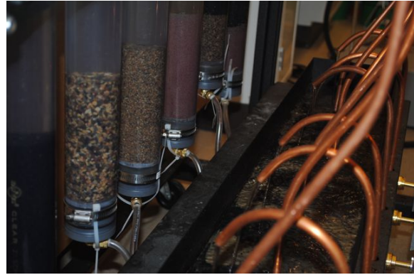
b) Filter columns with 4-inches of granular media in a range of particle sizes.
