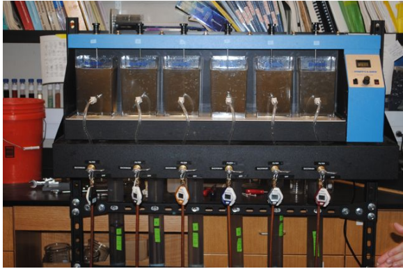
a) Preparation of turbid sediment-filled water for six different filter columns.
