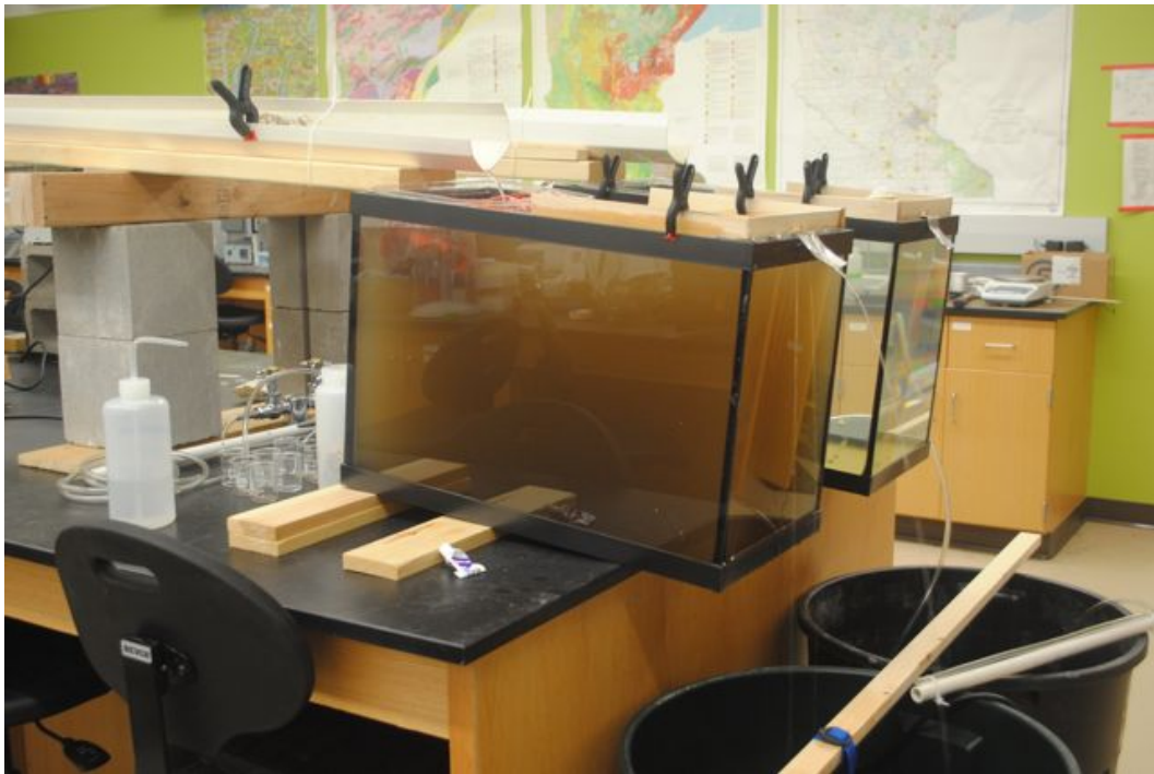
Figure 9. Twin 20-gallon sedimentation tanks, with orange snow fence submerged in inlet zone to reduce short-circuiting. Note two sampling locations: the end of channel/prior to inlet and the overflow weir of sedimentation tank.
