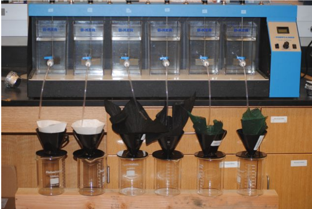
Figure 13. Membrane filtration apparatus with six parallel treatment lines, each consisting of mixing tank, valved delivery tubing, filter cone and filtrate collection beaker.
