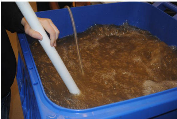
e) Mixing by air injection to 36-inch deep water in tank made from recycling bin.
