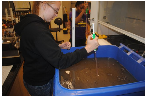
f) Sample collection for turbidity measurement.
