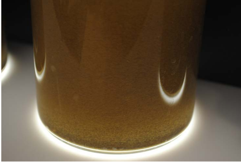
Figure 4. Floc formation (third jar from left in Figure 4) approximately 1 minute after flocculant dosing (end of rapid mix).
