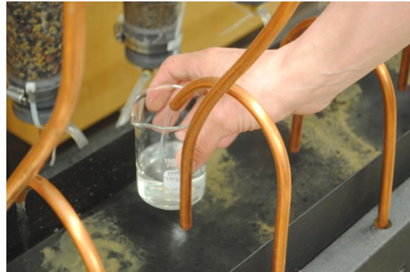
d) Sampling of flocculant-treated filtered water (turbidity ~10 NTU).
