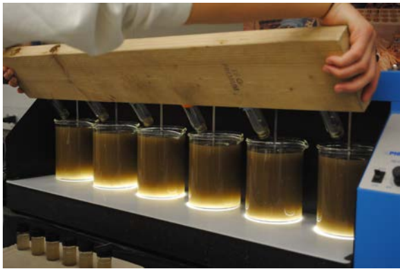
c) Simultaneous dosing of flocculants.
