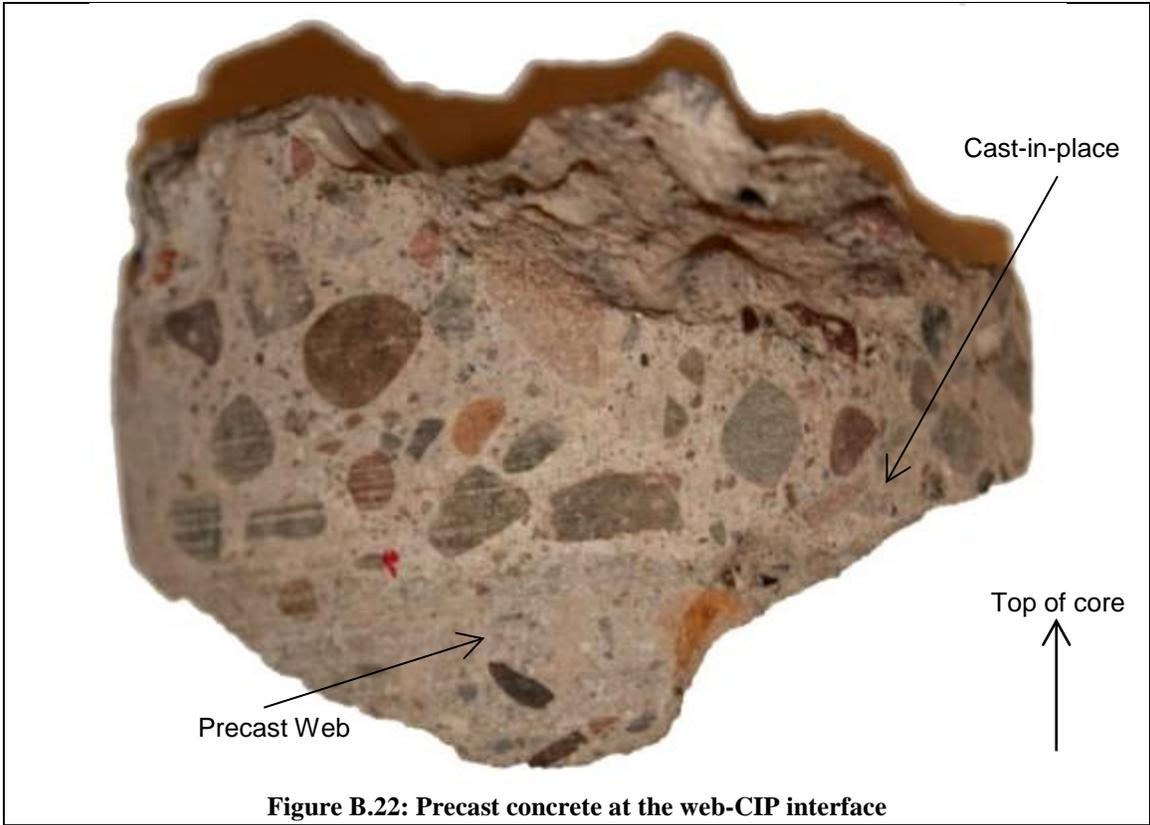
**Figure B.22: Precast concrete at the web-CIP interface**
