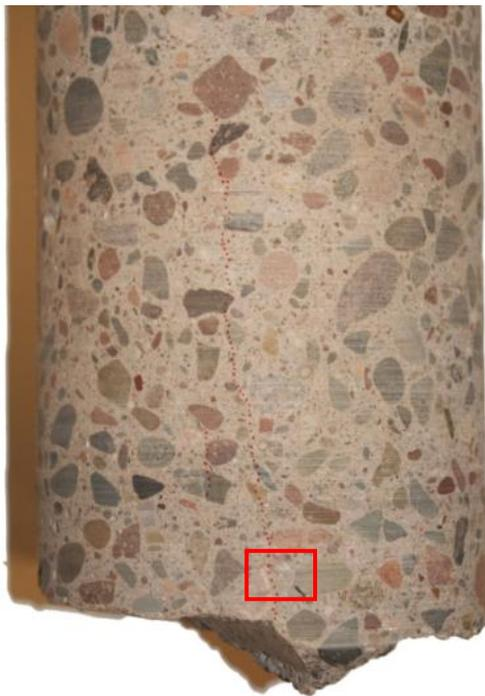
**Figure B.19: Reflective crack on the south face. There was a small crack adjacent to the reflective crack. Also note the uneven bottom surface due to differential camber.**
