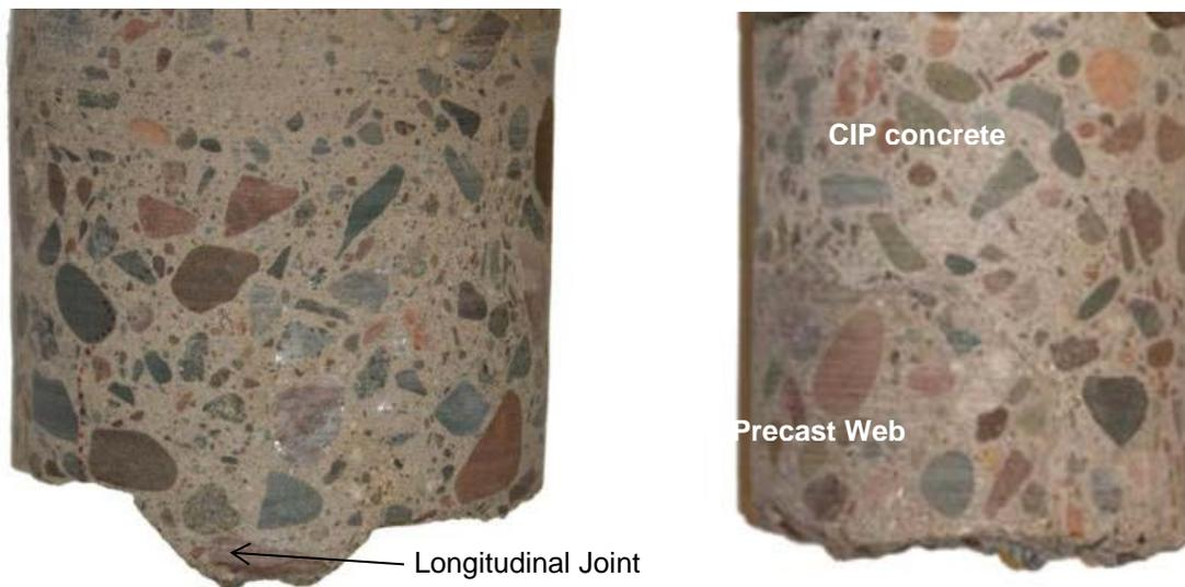
**Figure 3.12: Examples of a physically identifiable longitudinal joint (left) and web corner (right)**
