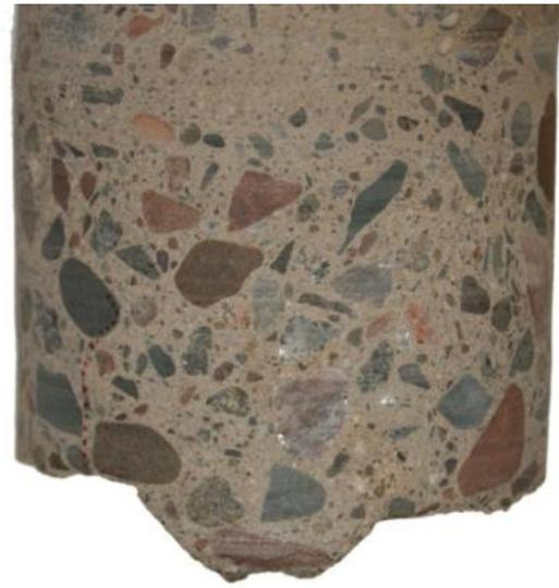
**Figure B.6: Visible camber difference in the joint of core 13004-2.**
