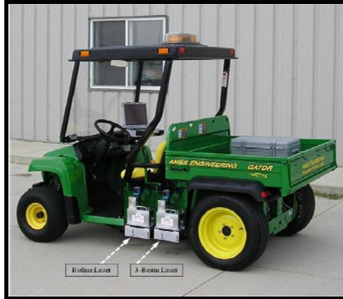
Figure 14. Lightweight Inertial Surface Analyzer (LISA) (ASTM E-950).
