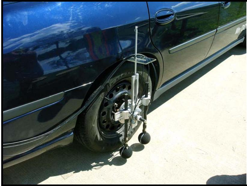
Figure 5. Chevrolet Impala with OBSI microphones attached.
