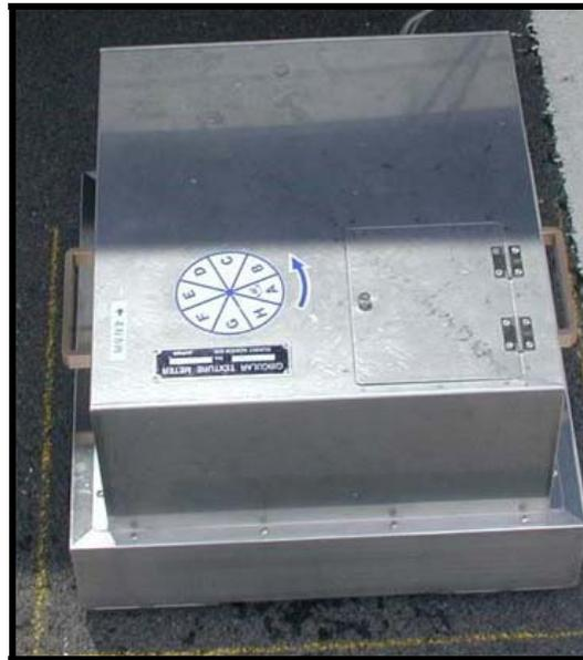
Figure 9. CTM Device (ASTM E-2157).
