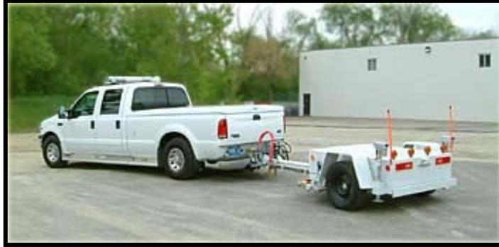
Figure 10. KJ Law (Dynatest 1295) Friction Trailer (ASTM E-274).
