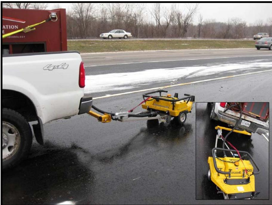
Figure 11. Findlay Irvine Grip Tester on loan from FHWA (ASTM E-274).
