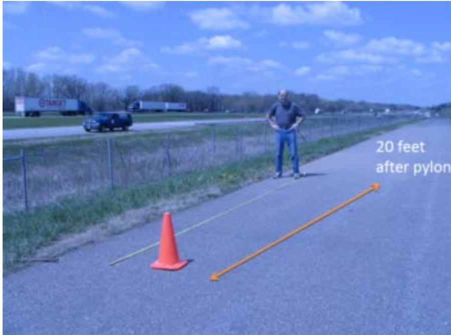
Figure 3.17 Conventional Applicator Delay
