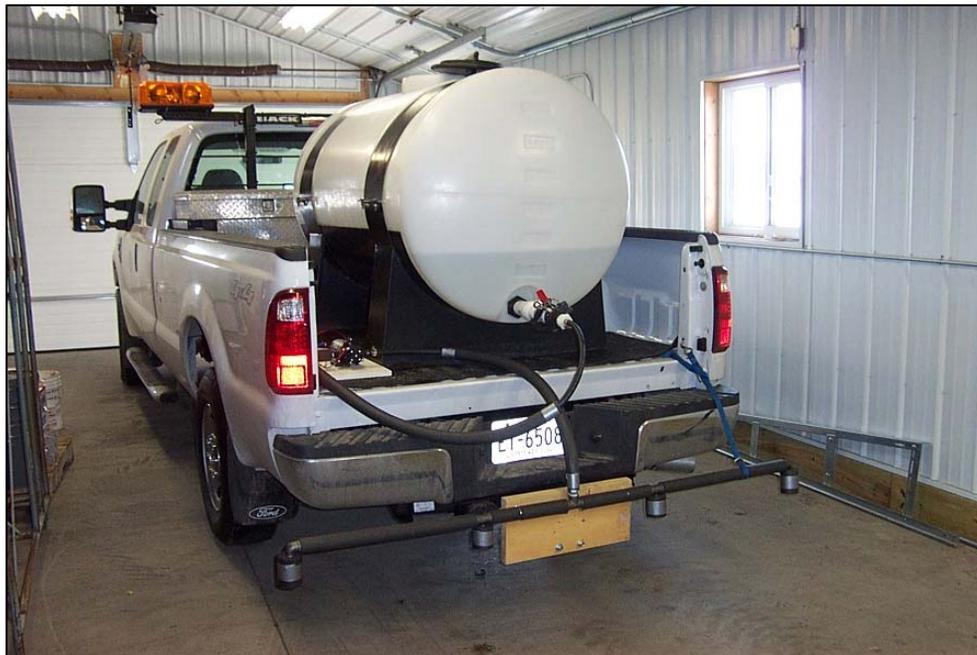
Figure 3.1 Pick-Up Truck Based Water Spray System
