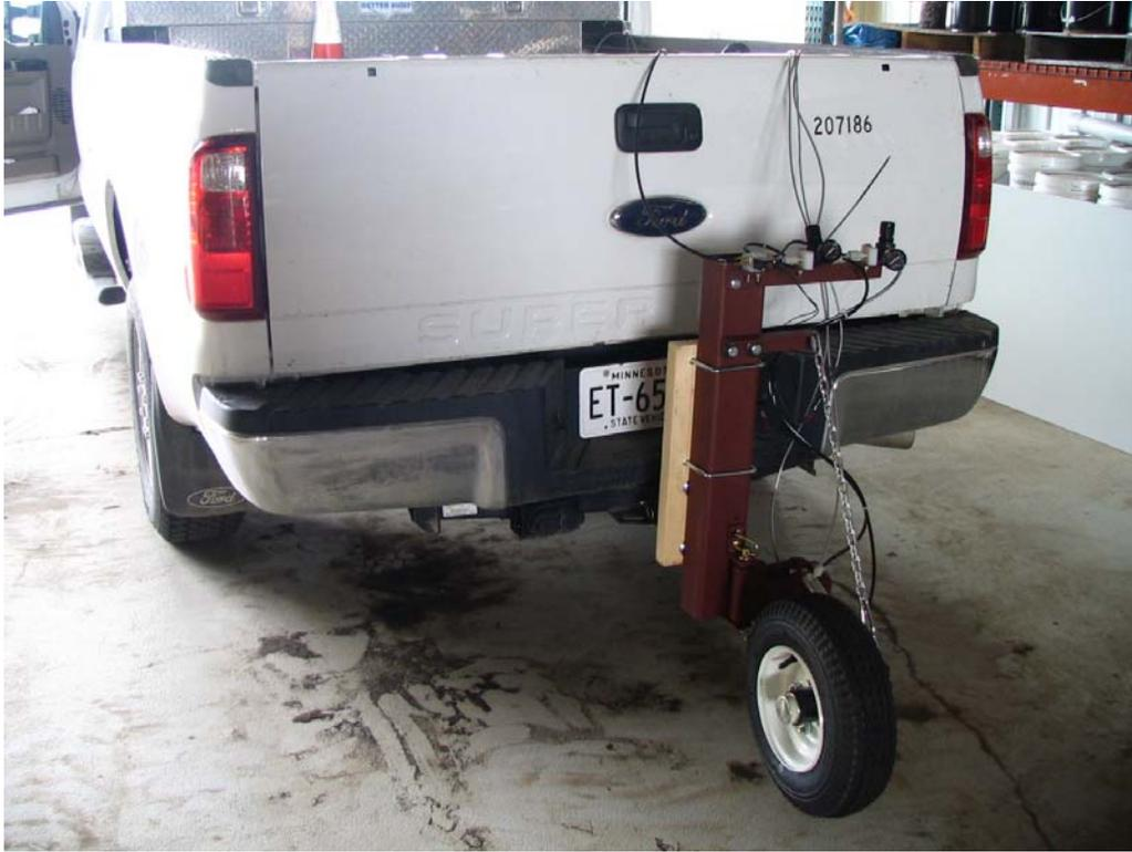
Figure 3.25 Friction Measurement System Installed on Pick-Up Truck
