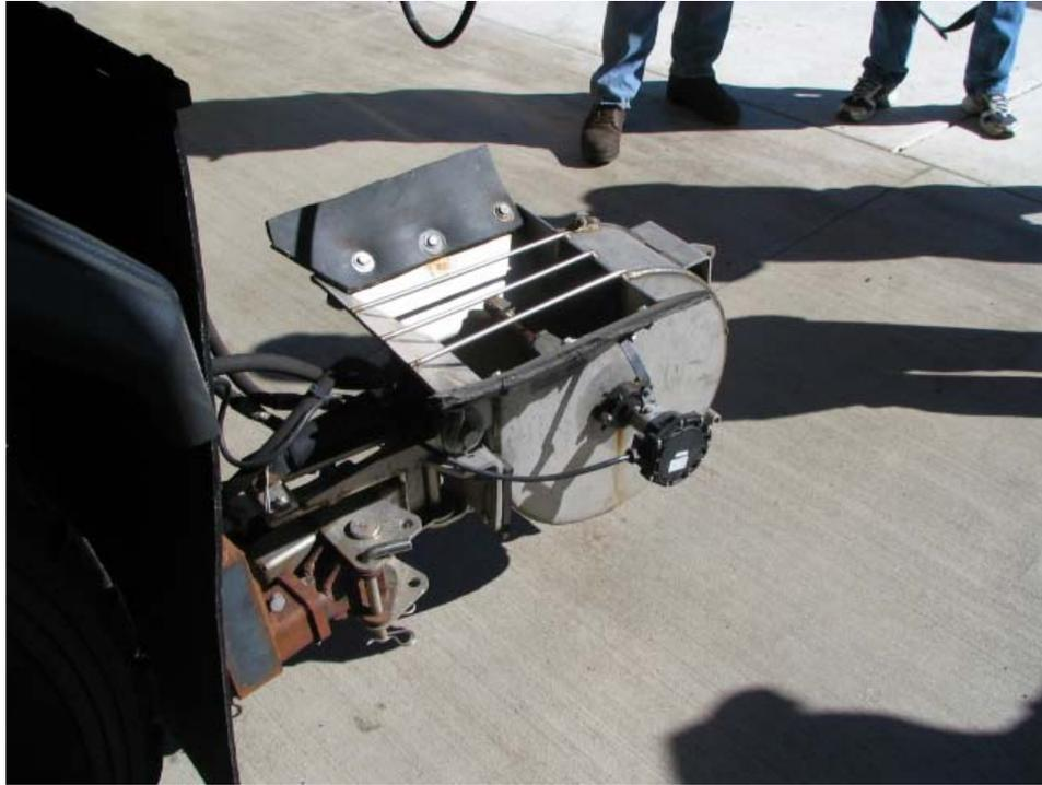
Figure 3.13 Zero Velocity Applicator
