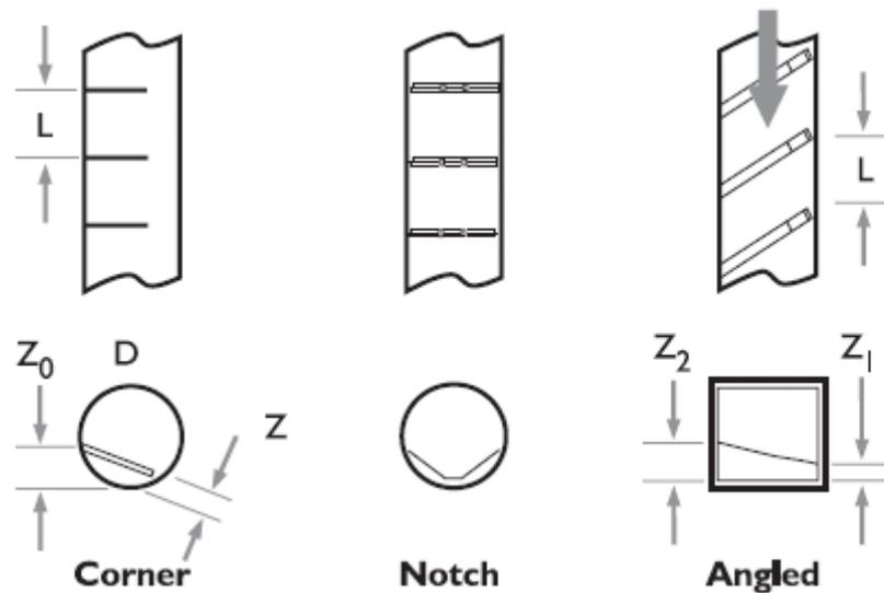
**Figure 4.4. Recommended styles of baffles for round and box culverts in Washington (Bates et al., 2003).**
