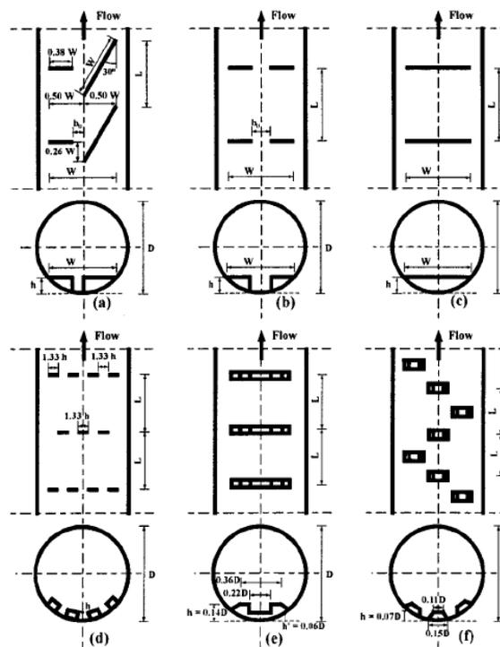
**Figure 4.3. (a) Offset; (b) slotted weir; (c) weir baffle; (d) spoiler; (e) Alberta fish weir (AFW); and (f) Alberta fish baffle (Ead et al., 2002).**
