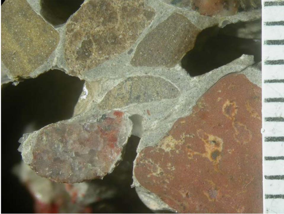
**Photo #11: Photomicrograph of the air voids in Sample #1. Note the lack of entrained air in the paste regions. Scale: 1 division = 1 mm**
