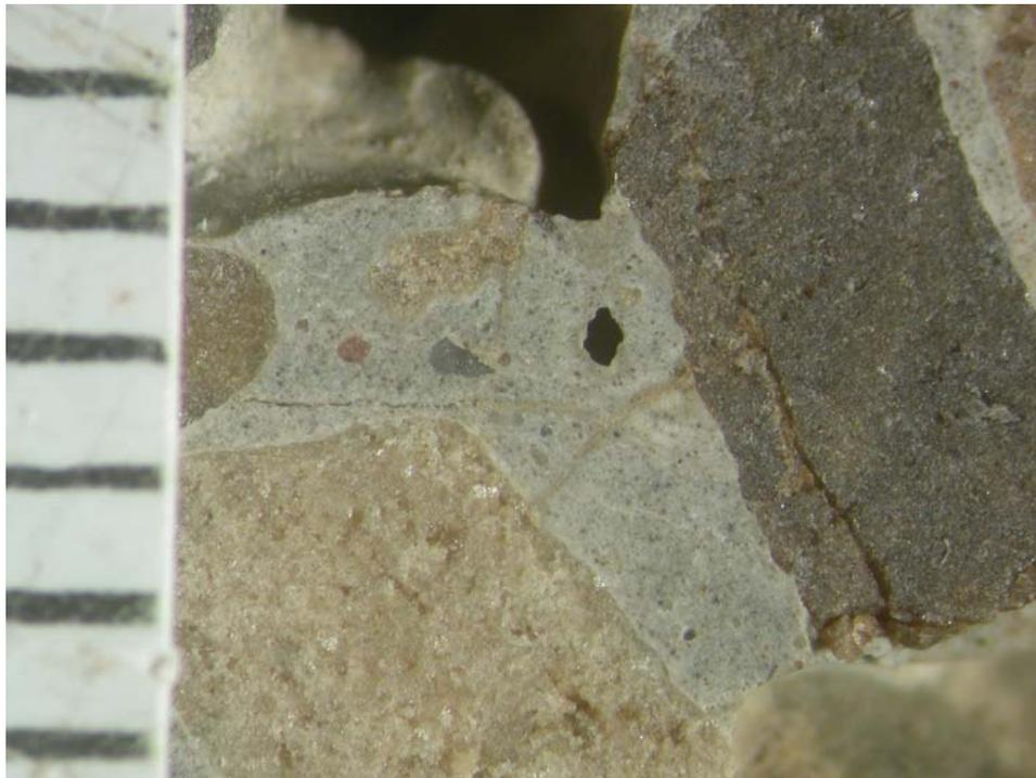
**Photo #12: Photomicrograph of the air voids in Sample #4. Note the lack of entrained air in the paste regions. Scale: 1 division = 1 mm**
