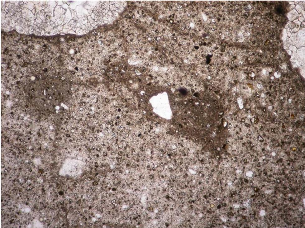
**Photo #8: Thin section photomicrograph of paste inhomogeneities in Sample #4.
