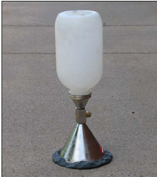
**FIGURE 7: In-situ drainability measurement device.**
