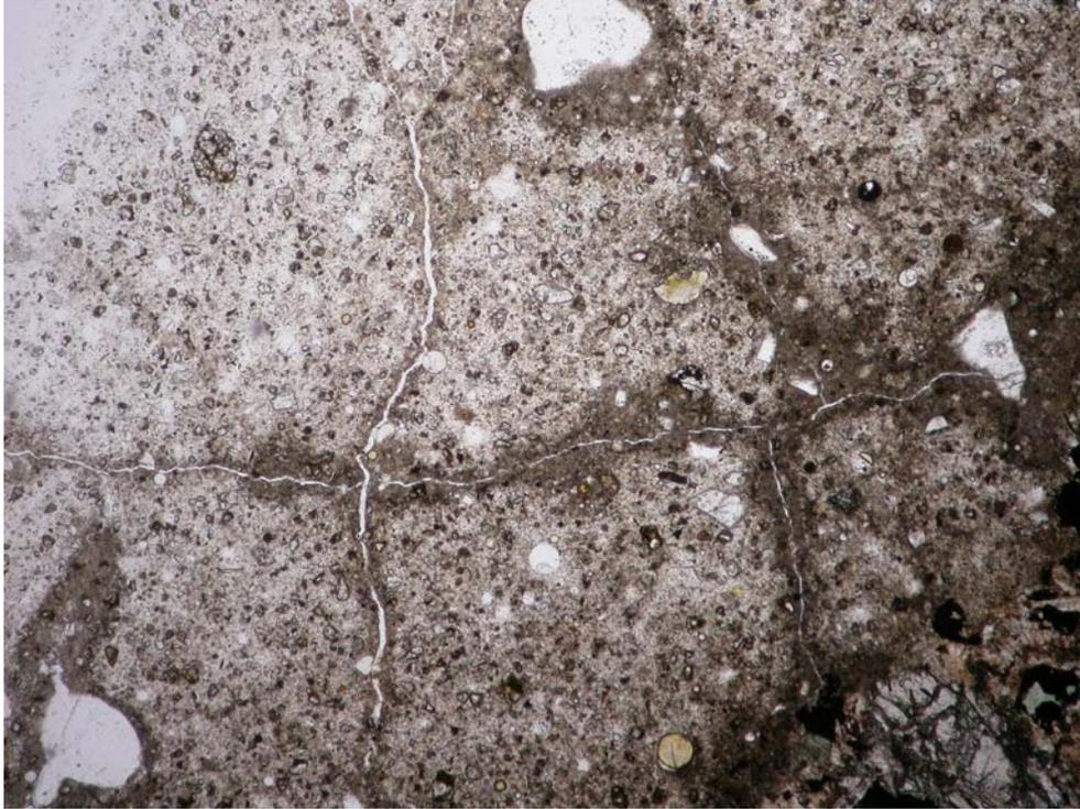
**Photo #9: Thin section photomicrograph of the extensive cracking in Sample #1.
