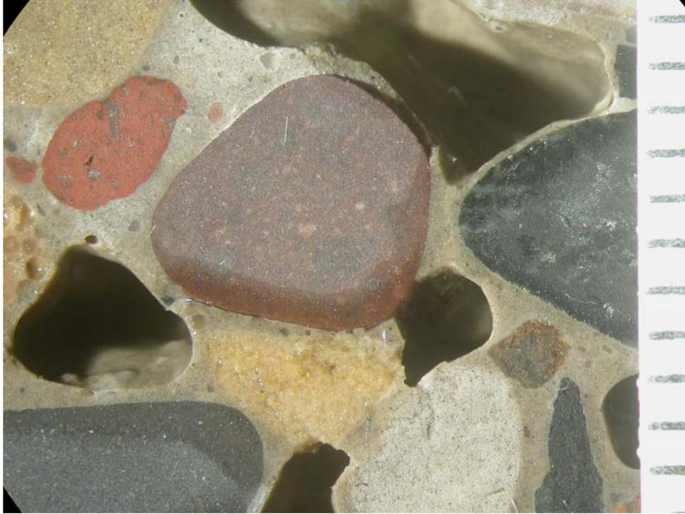
**Photo #13: Photomicrograph of the air voids in Sample #3. Note the lack of entrained air in paste regions. Scale: 1 division = 1 mm**
