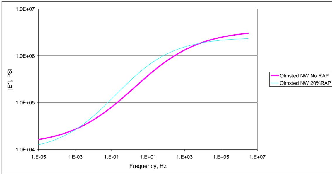
**Figure 27 –  $|E^*|$  master curve for Olmsted CR 112 non-wear course specimens; 58-34.**
