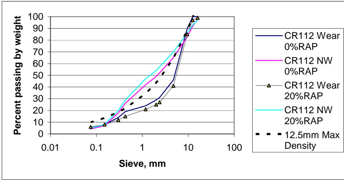
Figure 19 – Olmsted County extracted gradations.
