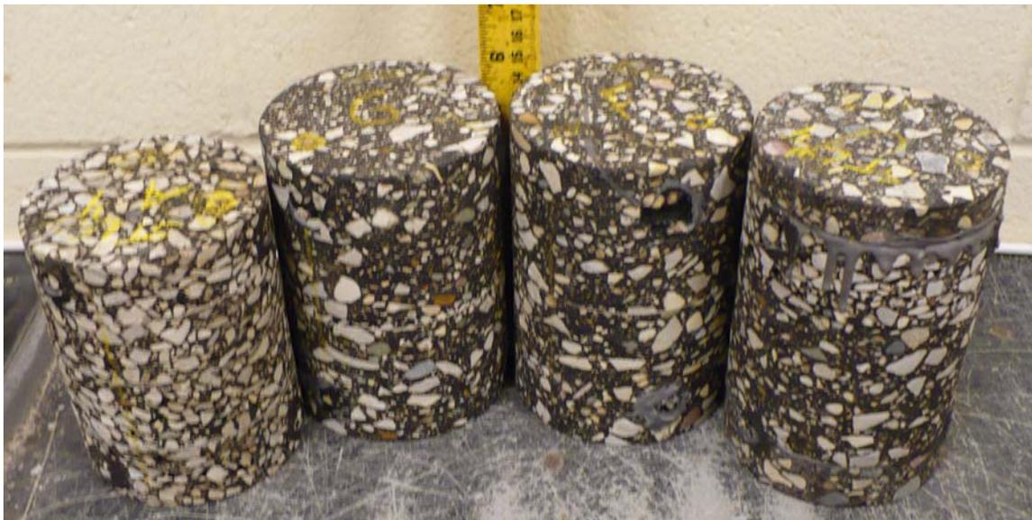
**Figure 15 –  $|E^*|$  specimen set from Olmsted CR 112 cores.**
