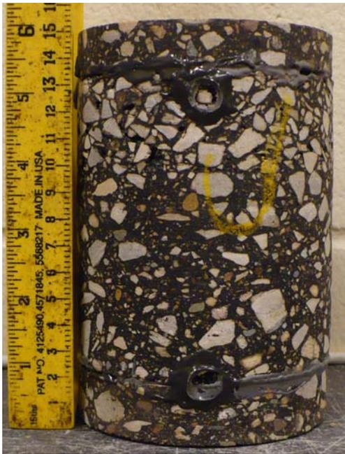
**Figure 17 – Full-depth |E\*| specimen from Olmsted CR 112 core.**
