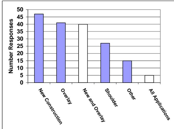
**Figure 6 – Use of RAP in pavement construction.**
