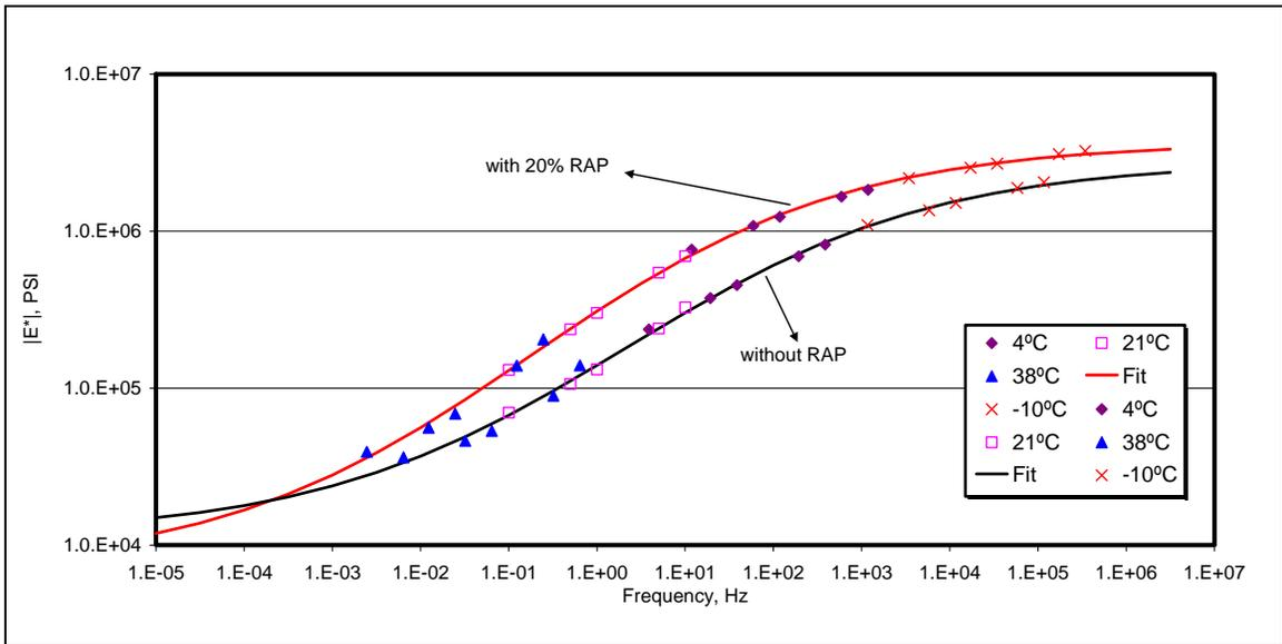
**Figure 25 –  $|E^*|$  master curve for Olmsted CR 112 full depth cores; 58-34.**
