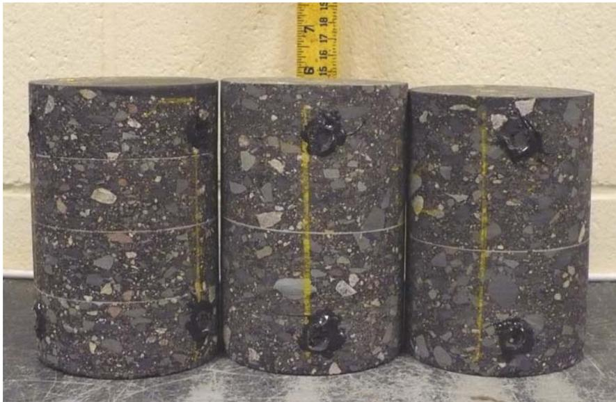
Figure 9 – One wear and two non-wear |E\*| specimens from St. Louis CR 4 cores.
