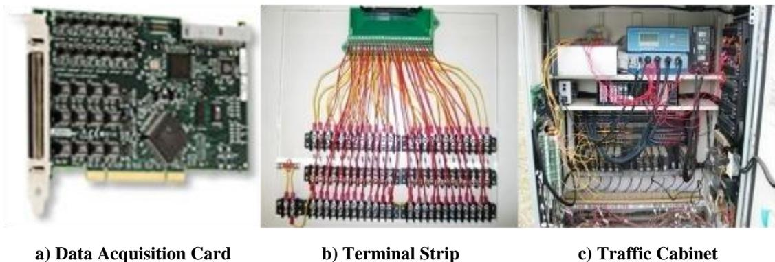
**Figure 3.3: Demonstration of the Traffic Data Collection Components.**
