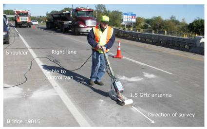
Researchers used ground penetrating radar (pictured), impedance spectroscopy and half-cell potential measurements in the field to evaluate the level of corrosion of the bars.
