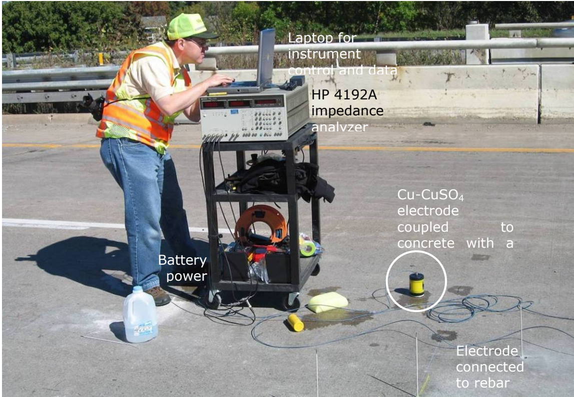
Figure 2.6 Electrical impedance spectroscopy setup and data acquisition system.
