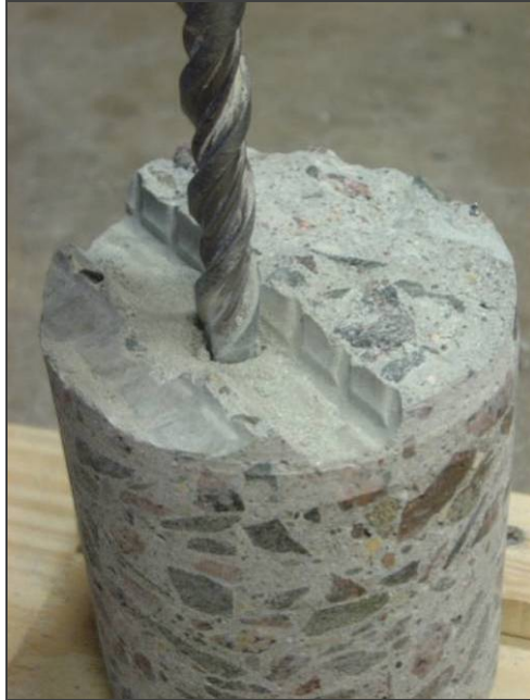
Figure 5.1 Concrete powder sample extraction by drilling.
