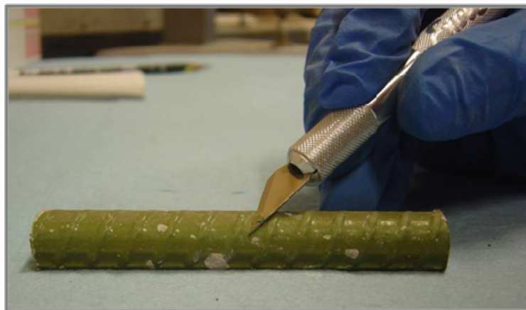
Figure 5.8 Dry knife adhesion test.
