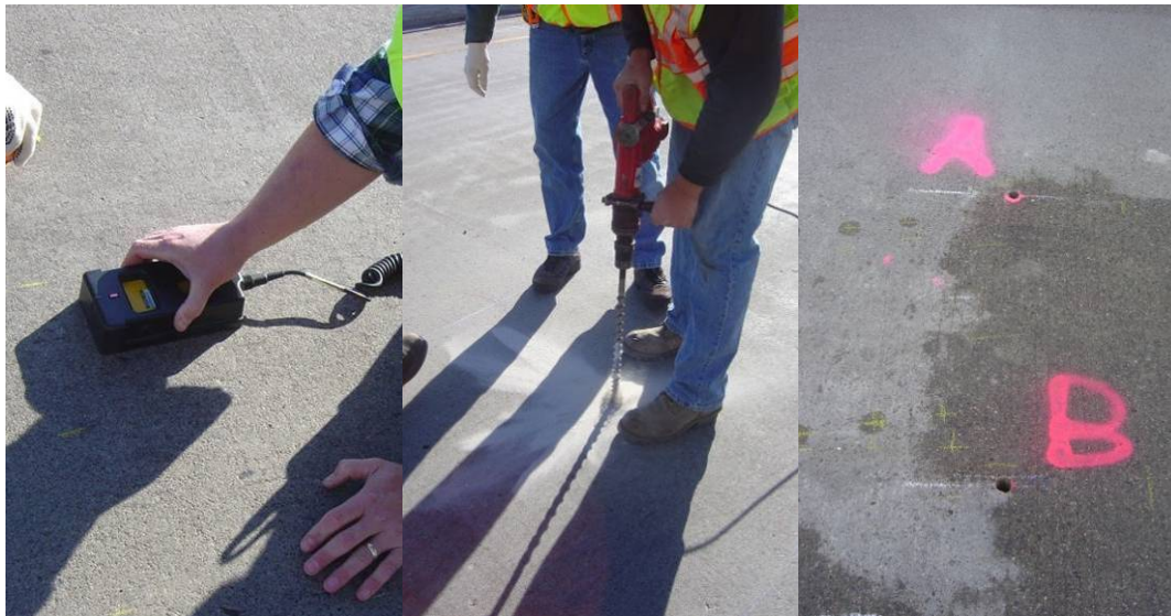
Figure 4.2 Connection to epoxy-coated bars.
