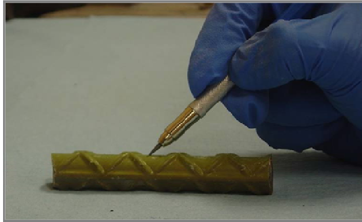
Figure 5.7 Pencil hardness test.
