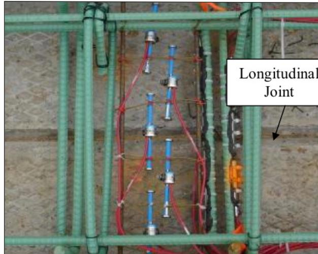
Strain gages were embedded in the concrete decking above the longitudinal joints of the bridge, providing researchers with data to study the development of cracks above the joints.
