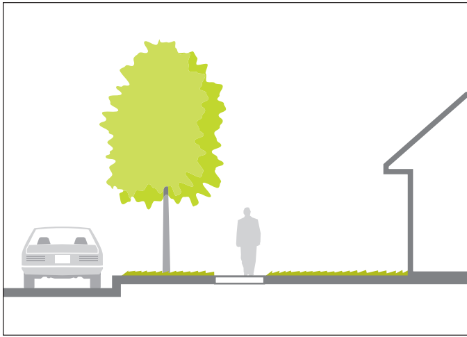
Figure 7.1. Adequate area between curb and sidewalk.
