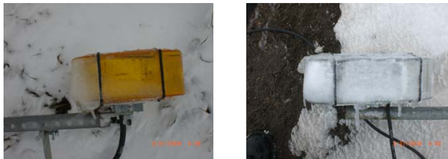
Figure 3. 9. Photographs of standard strobe and Whelen LED after heavy snow conditions
