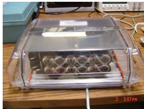
Figure 1. 6. Photo of one of the LED strobes from PSE used in this study
