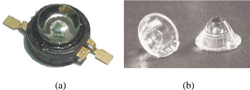
Figure 1. 8. Image of a typical (a) LED emitter and (b) lens used in the LED strobes [8]
