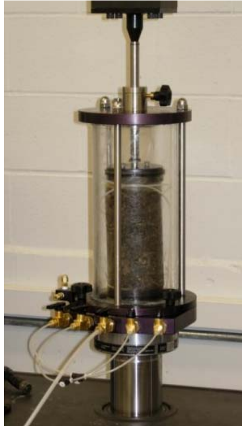
Figure 4.1. Emulsion sample in triaxial cell.
