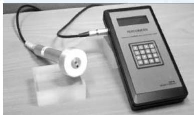
Researchers used a percometer to measure dielectric constants in order to find correlations with pavement and soil material properties.
