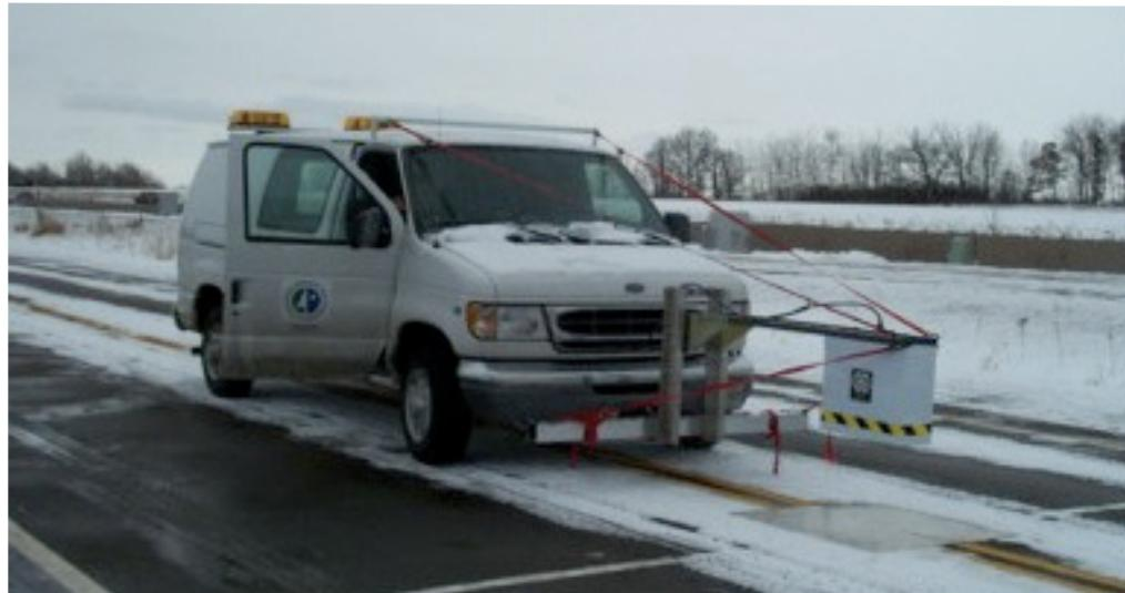
GPR is mounted on a van and gathers pavement structural data, such as thickness, at 50 mph so workers don't need to close traffic lanes to cut out multiple pavement samples.
