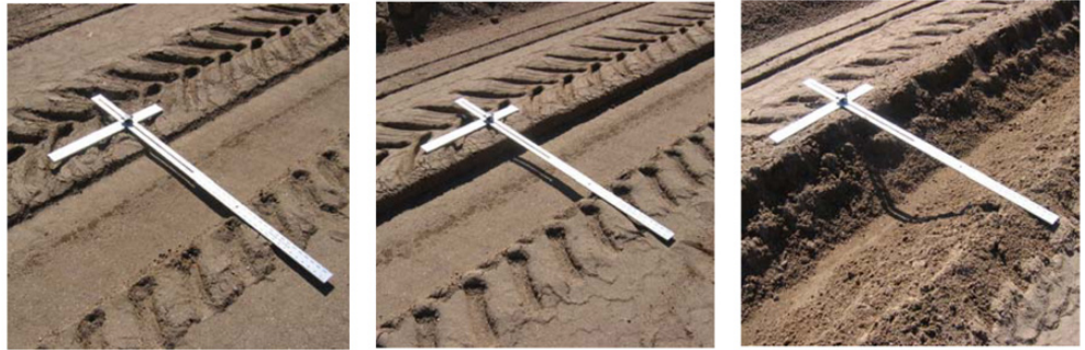
Evaluating test-rolled soil using current test rolling procedures: passing inspection (left), near failing (center) and failing (right).
