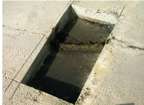
Figure 10 Ridge of fine material in the upper HMA layer of test pit No. 2, located at the centerline.
