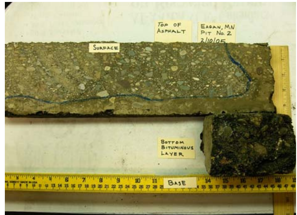
Figure 14 Eagan pit No. 2 with moist regions highlighted.
