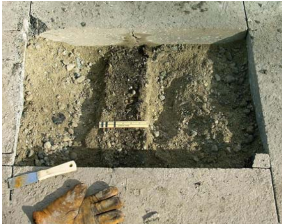
Figure 9 Frozen lens at top of test pit No. 1, located at the outer edge of the lane.
