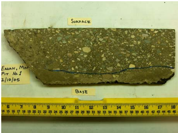
Figure 13 Eagan pit No. 1 with moist regions highlighted.
