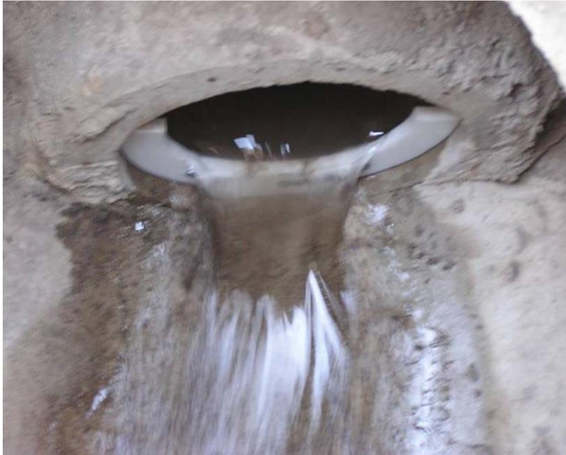
**Figure C.10:** Pre-calibrated 12” circular weir installed downstream of the Vortechs System. Pressure transducer and transducer anchoring not shown. This weir location provided free outfall conditions at all flow rates due to the favorable gradient across the manhole and downstream storm drain system.
