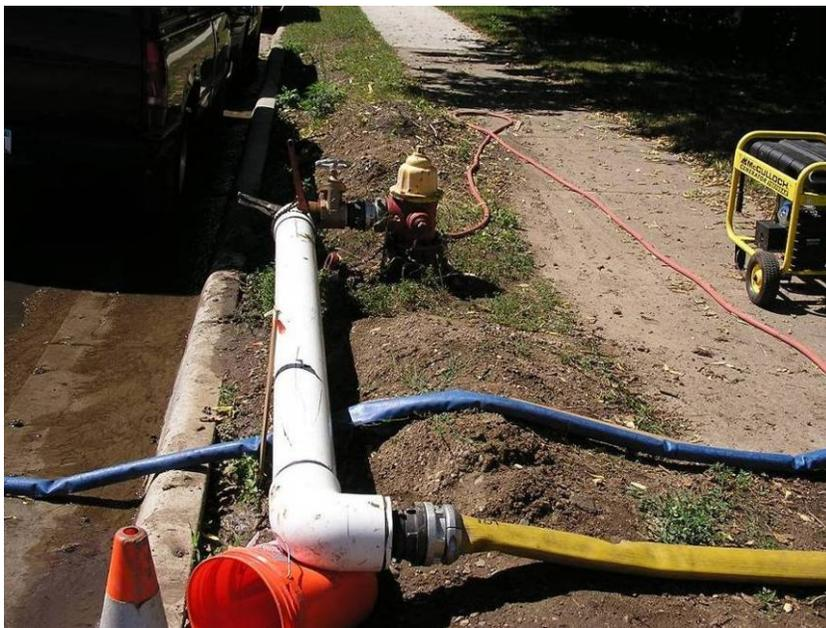
**Figure C.11:** Upstream portion of influent delivery system from the water source at the hydrant to the first reach of 4” fire hose in the foreground.
