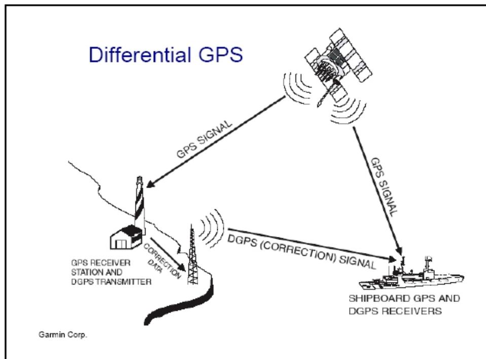
**Figure 3.2** Illustration of “real time” differential correction.
