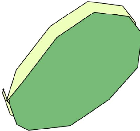
**Figure 3.3** *An example of the spatial impact of differential correction. The differentially corrected polygon (dark or dark green) is shifted slightly southeast compared to the uncorrected polygon (light or light green).*
