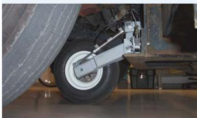
Because the measurement system's small wheel is set at an angle, it receives a lateral force corresponding to the road's surface friction.
