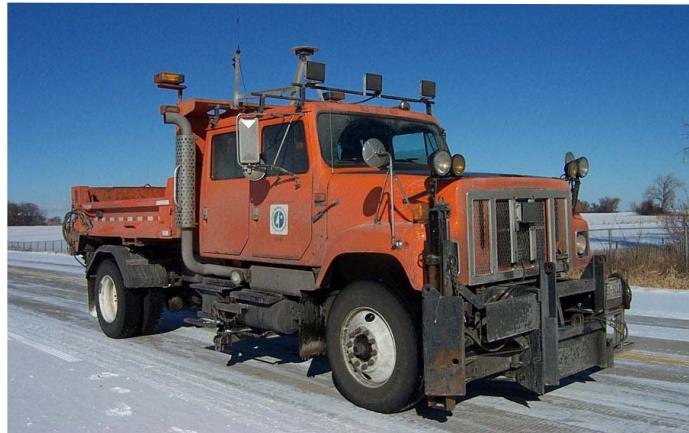
The new measurement system can be fitted on full-size snowplows and delivers real-time surface friction readings to an automatic control system that dispenses deicing chemicals.
