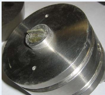
Bender elements are thin pieces of piezo-ceramic material that can be used to measure seismic wave velocities.
