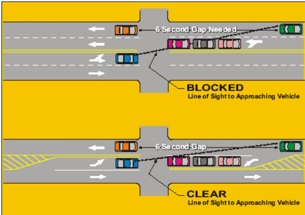
Figure 4.3: Effects of off-set left-turn design on sight distance
