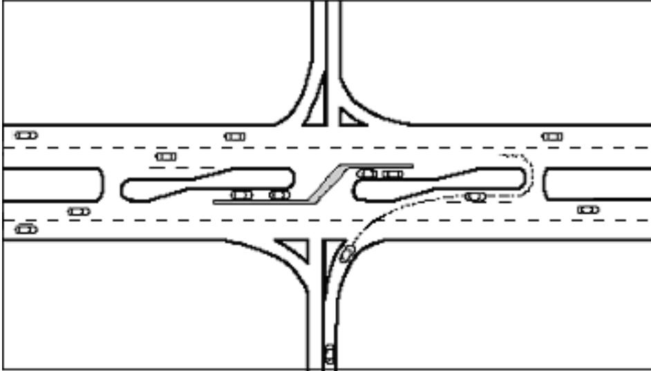
Figure 4.9: Directional Median Opening
