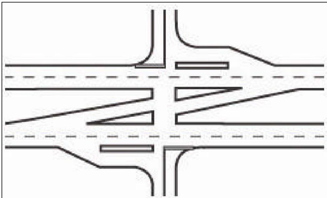
Figure 4.4: Intersection with offset right and left turn lanes
