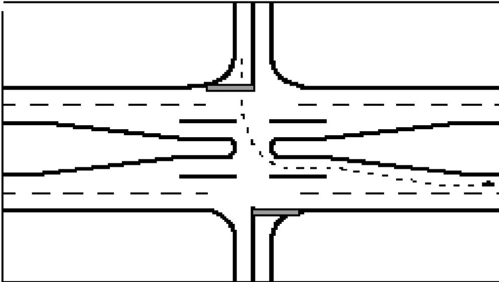
Figure 4.1: Median left-turn acceleration lane
