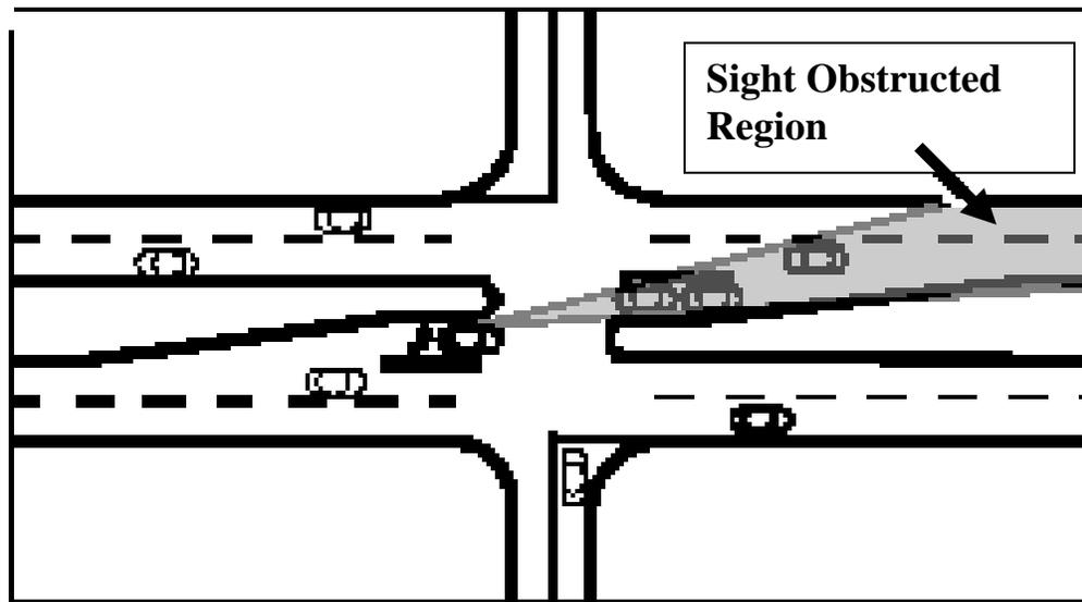
Figure 4.2: Obstructed Sight distance due to opposing left-turning vehicles
