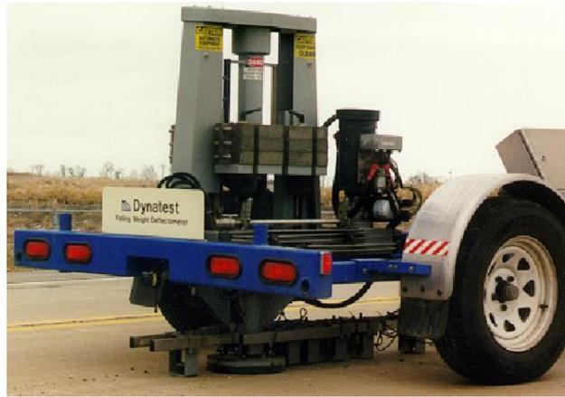
A falling-weight deflectometer tests stiffness by dropping a weight onto a loading plate on the pavement surface and recording the pavement and base response with sensors.
