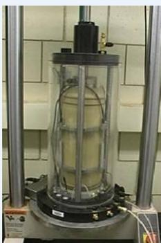
Laboratory stiffness testing involves recording the response of a sample of base material in a pressure vessel to a series of loads.
