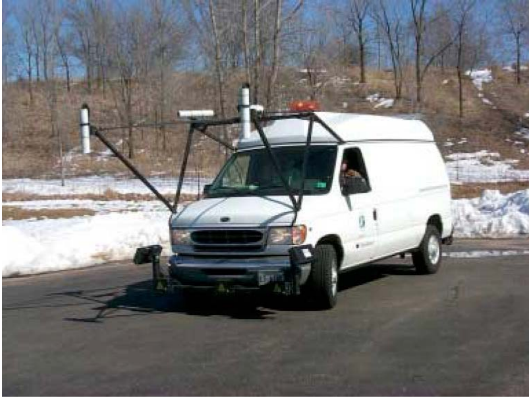
Figure 3: Pathway Services, Inc Video Inspection Vehicle (VIV) (4).
