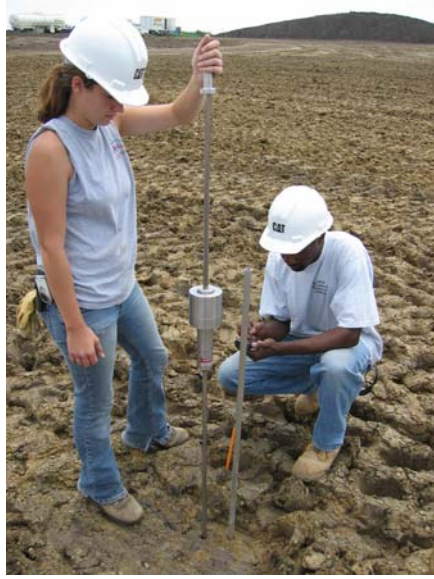
Figure 2.11. Strength determination using dynamic cone penetrometer
