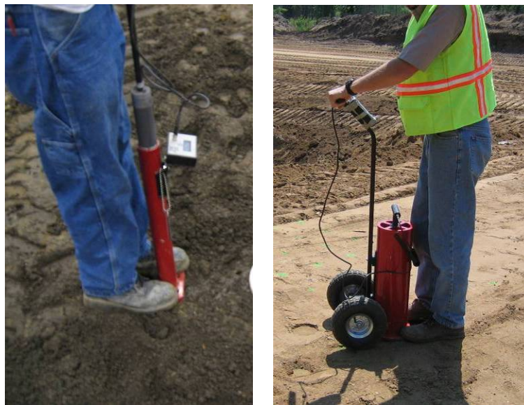
Figure 2.12. Strength determination using Clegg impact testers: 4.5-kg (left) and 20-kg (right)
