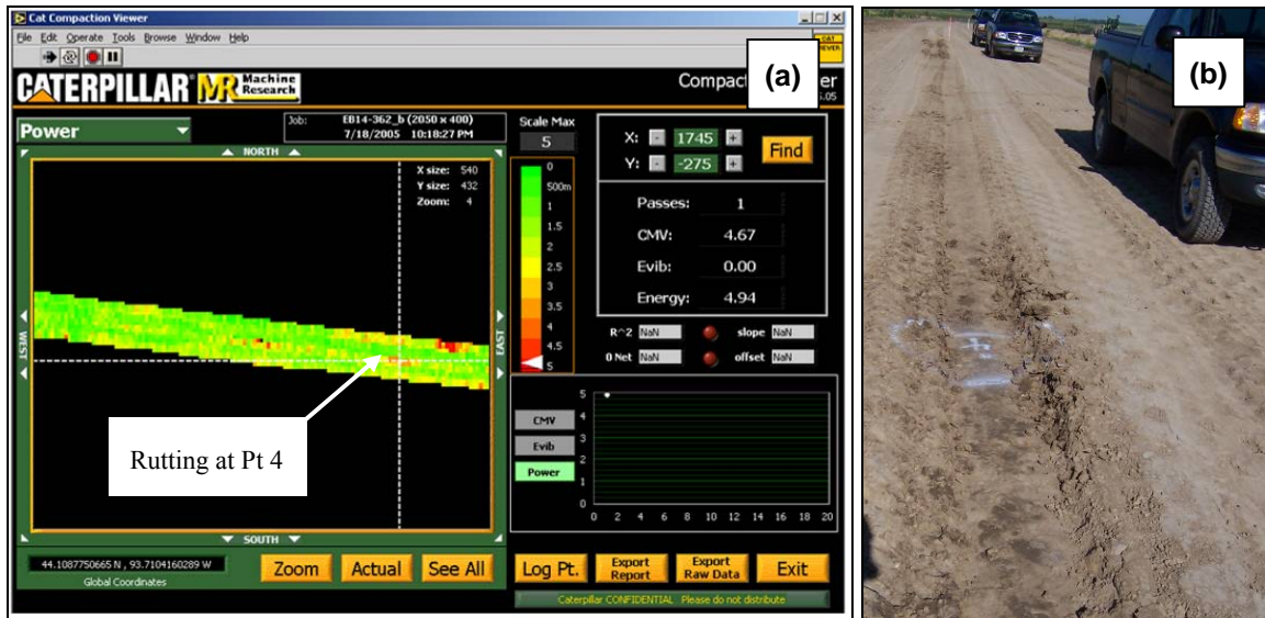
Figure 3.10. Eastbound STA 362 to 385: (a) compaction monitor view (viewing area 165 x 132 m) and (b) rutting at Point 4
