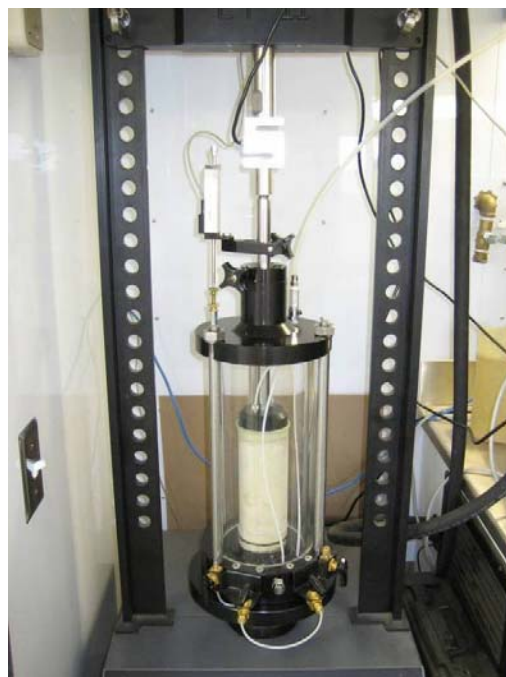
Figure 2.7. Resilient modulus triaxial chamber setup
