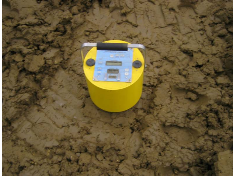
Figure 2.13. Modulus determination using soil stiffness gauge
