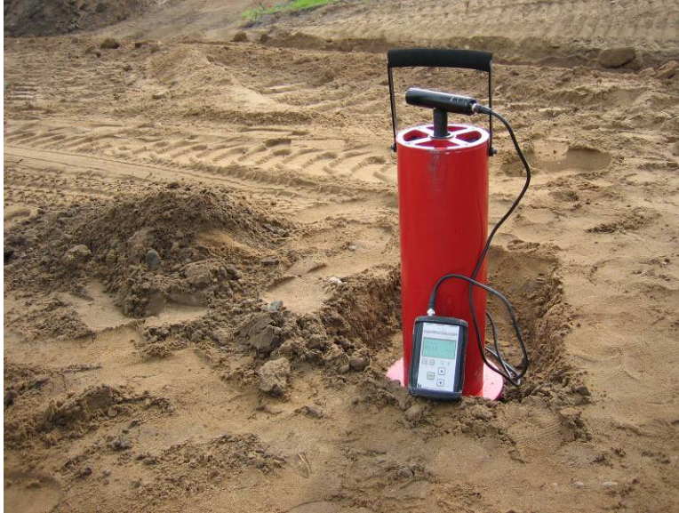
Figure 5.25. Clegg impact tester (20-kg) at 195-mm depth
