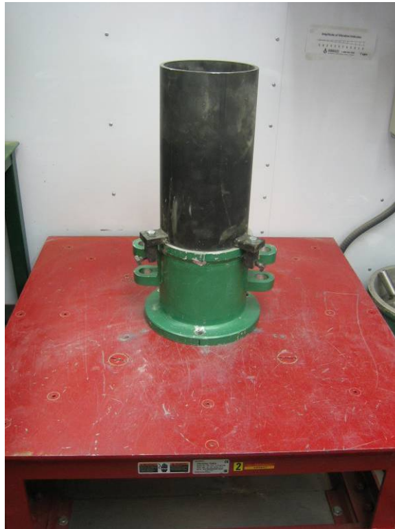
Figure 2.4. 152 mm (6 inch) diameter compaction mold and vibratory table
