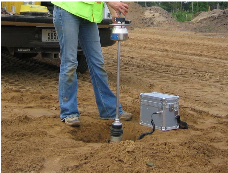
Figure 5.26. 200-mm Zorn ZFG light weight deflectometer at 220-mm depth
