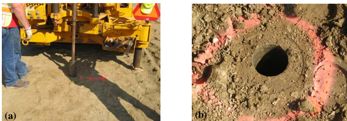
Figure 9.10. Figures showing tube extraction process (a) Mn/DOT drill rig pushing a 4 inch diameter shelly tube, and (b) LWD and tube locations
