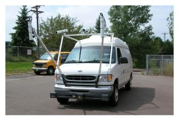
IRI smoothness data can be collected using high-speed, vanmounted laser systems, which excel at detecting the types of roughness experienced by vehicle occupants.
