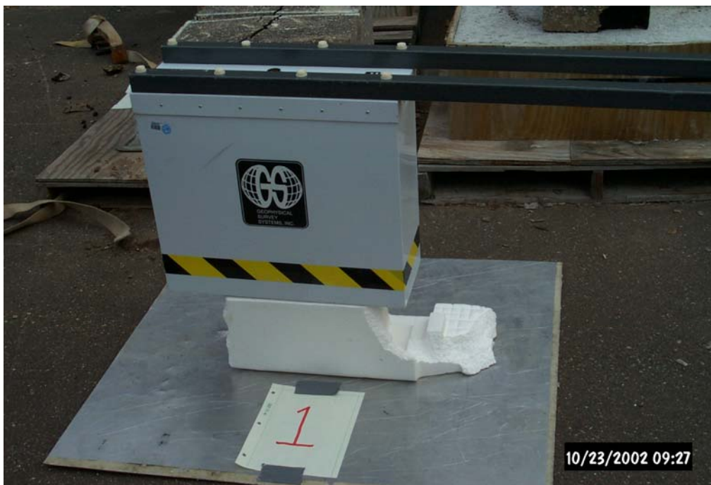
Figure 3-1 Configuration #1 Setup – 1000 MHz Antenna
