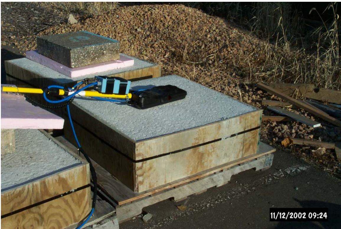
Figure 3-3 Configuration #2 Setup – 1000 MHz Antenna
