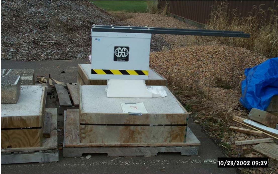
Figure 3-3 Configuration #2 Setup – 1000 MHz Antenna
