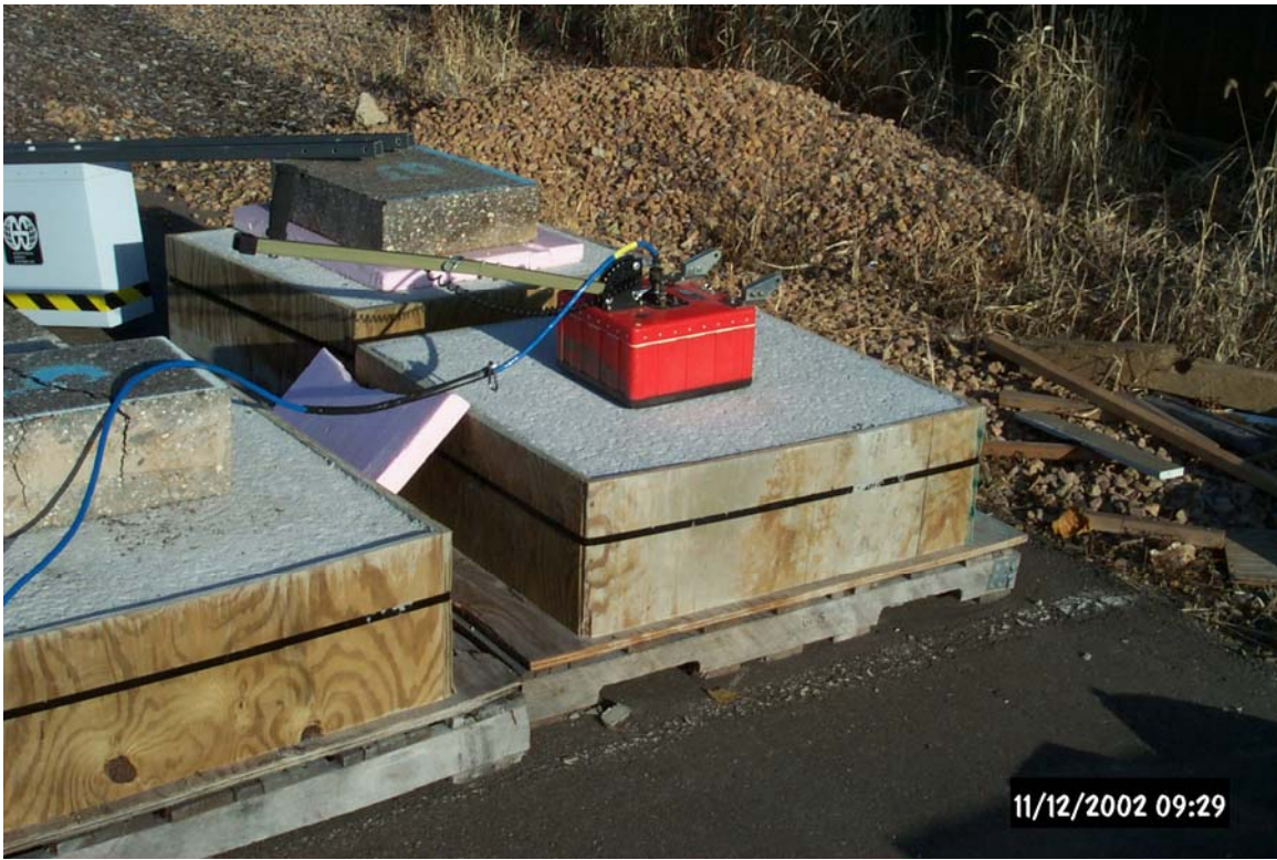
Figure 3-5 Configuration #2 Setup – 400 MHz Antenna
