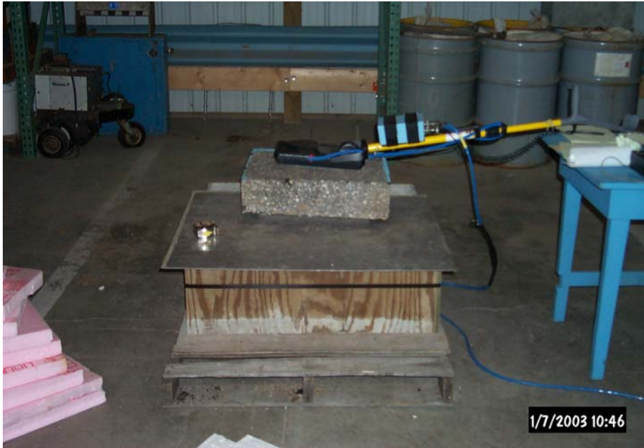
Figure 3-14 Laboratory Setup for Air Void Thickness Study
