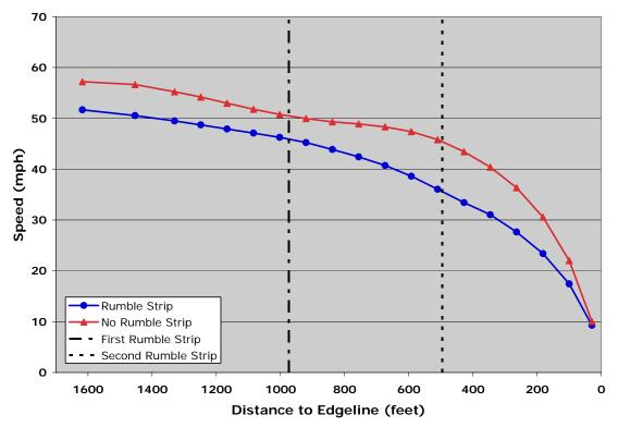
Figure 3.9: Commercial Vehicle/Heavy Truck Category—Mean Speeds on the Approach to *Obscure/Visible* Intersections *With Rumble Strips* and *Without Rumble Strips*.
