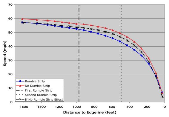
Figure 3.5: SUV/Pick-Up Truck/Van Category—Mean Speeds on the Approach to *Obscure/Visible* Intersections *With Rumble Strips* and *Without Rumble Strips*.
