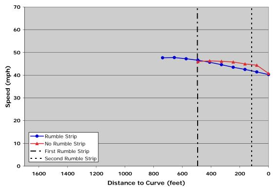
Figure 3.19: Commercial Vehicle/Heavy Truck Category—Mean Speeds on the Approach to *Horizontal Curve* Intersections *With Rumble Strips* and *Without Rumble Strips*.
