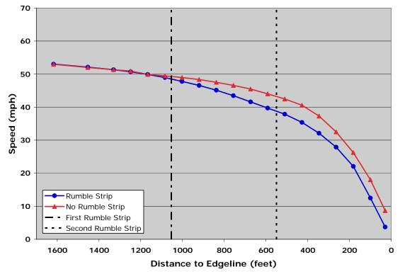
Figure 3.3: Commercial Vehicle/Heavy Truck Category—Mean Speeds on the Approach to *Obscure Both* Intersections *With Rumble Strips* and *Without Rumble Strips*.
