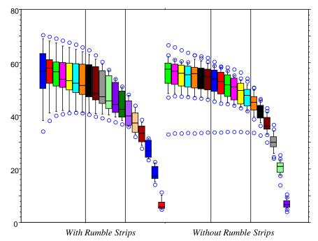
Figure 3.8: Passenger Car Category—Boxplots of Individual Mean Speeds in the Segments on the Approach to *Obscure/Visible* Intersections *With Rumble Strips* and *Without Rumble Strips*.
