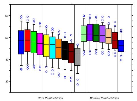
Figure 3.18: SUV/Pick-Up Truck/Van Category—Boxplots of Individual Mean Speeds in the Segments on the Approach to *Horizontal Curve* Intersections *With Rumble Strips* and *Without Rumble Strips*.
