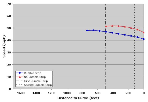
Figure 3.17: SUV/Pick-Up Truck/Van Category—Mean Speeds on the Approach to *Horizontal Curve* Intersections *With Rumble Strips* and *Without Rumble Strips*.
