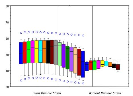
Figure 3.24: Commercial Vehicle/Heavy Truck Category —Boxplots of Individual Mean Speeds in the Segments on the Approach to *Vertical Curve* Intersections *With Rumble Strips* and *Without Rumble Strips*.
