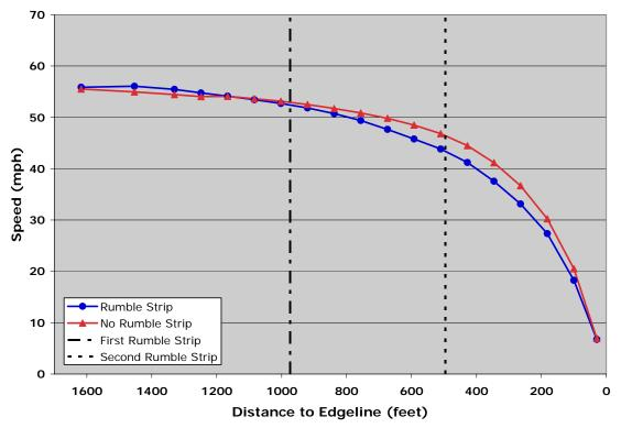
Figure 3.7: Passenger Car Category—Mean Speeds on the Approach to *Obscure/Visible* Intersections *With Rumble Strips* and *Without Rumble Strips*.
