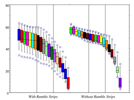
Figure 3.10: Commercial Vehicle/Heavy Truck Category—Boxplots Mean Speeds on the Approach to *Obscure Both* Intersections *With Rumble Strips* and *Without Rumble Strips*.
