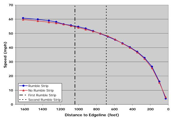
Figure 3.13: Passenger Car Category—Mean Speeds on the Approach to Visible Both Intersections With Rumble Strips and Without Rumble Strips.
