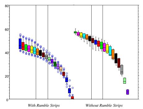
Figure 3.16: Commercial Vehicle/Heavy Truck Category—Boxplots of Individual Mean Speeds in the Segments on the Approach to *Visible Both* Intersections *With Rumble Strips* and *Without Rumble Strips*.
