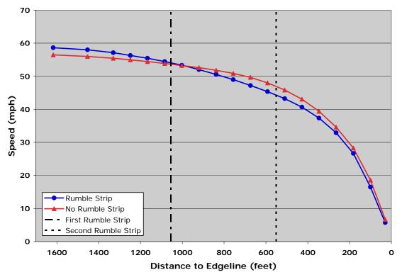
Figure 3.1: SUV/Pick-Up Truck/Van Category—Mean Speeds on the Approach to *Obscure Both* Intersections *With Rumble Strips* and *Without Rumble Strips*.
