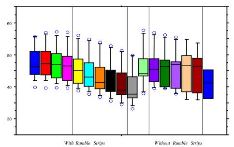
Figure 3.20: Commercial Vehicle/Heavy Truck Category —Boxplots of Individual Mean Speeds in the Segments on the Approach to *Horizontal Curve* Intersections *With Rumble Strips* and *Without Rumble Strips*.
