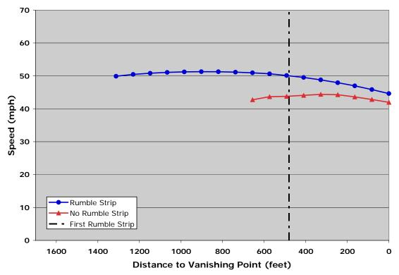
Figure 3.23: Commercial Vehicle/Heavy Truck Category—Mean Speeds on the Approach to *Vertical Curve* Intersections *With Rumble Strips* and *Without Rumble Strips*.
