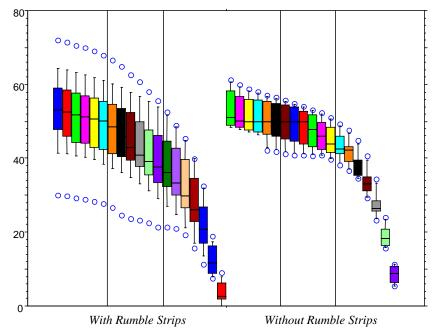
Figure 3.4: Commercial Vehicle/Heavy Truck Category—Boxplots of Individual Mean Speeds in the Segments on the Approach to *Obscure Both* Intersections *With Rumble Strips* and *Without Rumble Strips*.
