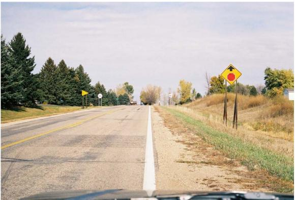
Photographs #116 & 117 (Reel #6, 11A & 12 A) (from South, looking North): first rumble strip and warning in view. [Note: at this point driver approaching intersection has just crossed railway track.]
