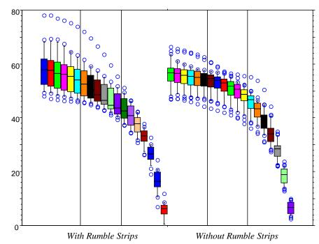
Figure 3.2: SUV/Pick-Up Truck/Van Category—Boxplots of Individual Mean Speeds in the Segments on the Approach to *Obscure Both* Intersections *With Rumble Strips* and *Without Rumble Strips*.
