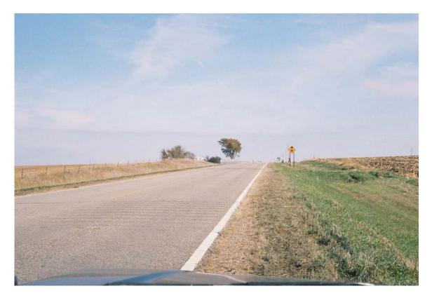
Photograph #149 (Reel #7, 20A) (from West, looking East): first rumble strip and warning sign in view.
