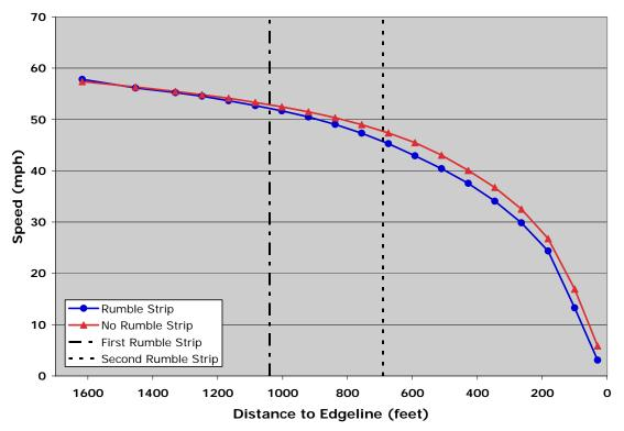
Figure 3.11: SUV/Pick-Up Truck/Van Category—Mean Speeds on the Approach to *Visible/Both* Intersections *With Rumble Strips* and *Without Rumble Strips*.
