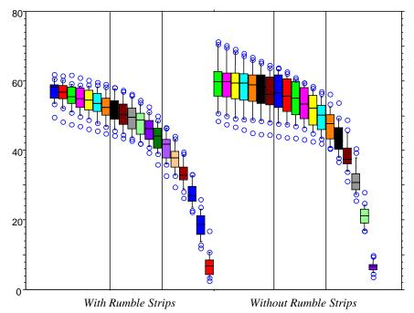
Figure 3.6: SUV/Pick-Up Truck/Van Category—Boxplots of Individual Mean Speeds in the Segments on the Approach to *Obscure/Visible* Intersections *With Rumble Strips* and *Without Rumble Strips*.
