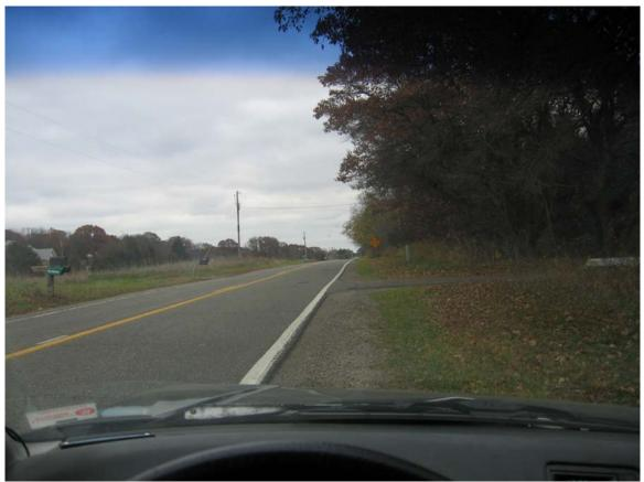
Photograph #470 (Reel #E1, 19) (from North, looking South): *no rumble strip*; warning sign in view (just *before* crest of vertical curve).
