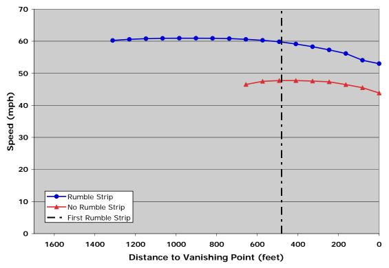
Figure 3.21: Passenger Car Category—Mean Speeds on the Approach to *Vertical Curve* Intersections *With Rumble Strips* and *Without Rumble Strips*.
