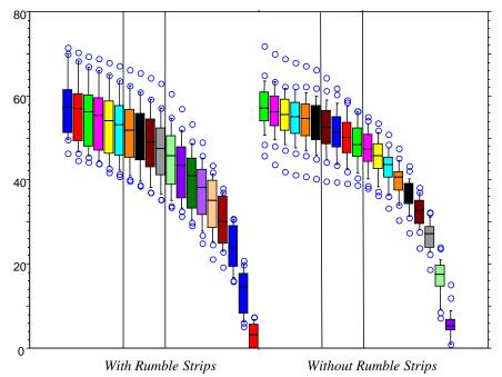
Figure 3.12: SUV/Pick-Up Truck/Van Category—Boxplots of Individual Mean Speeds in the Segments on the Approach to *Visible Both* Intersections *With Rumble Strips* and *Without Rumble Strips*.
