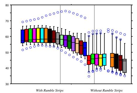
Figure 3.22: Passenger Car Category—Boxplots of Individual Mean Speeds in the Segments on the Approach to *Vertical Curve* Intersections *With Rumble Strips* and *Without Rumble Strips*.
