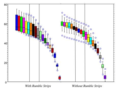
Figure 3.14: Passenger Car Category—Boxplots of Individual Mean Speeds in the Segments on the Approach to *Visible Both* Intersections *With Rumble Strips* and *Without Rumble Strips*.
