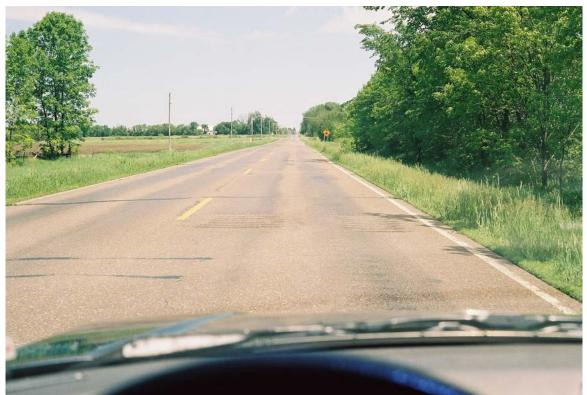
Photograph #247 (Reel #12, 9A) (from West, looking East): first *of four* sets of rumble strips and warning sign in view; also STOP AHEAD on road (though barely visible in this photograph).
