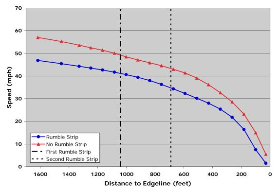
Figure 3.15: Commercial Vehicle/Heavy Truck Category—Mean Speeds on the Approach to *Visible Both* Intersections *With Rumble Strips* and *Without Rumble Strips*.
