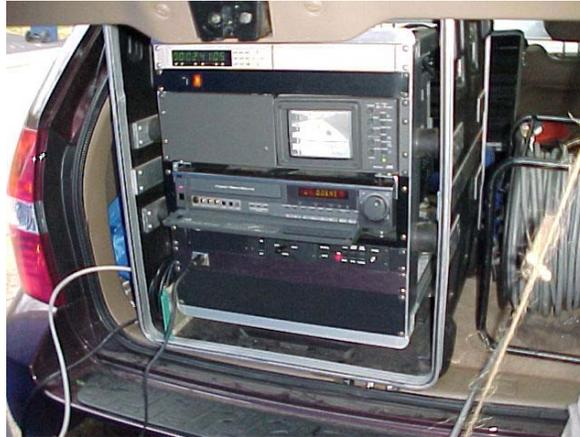
**Figure 5.2: Video recording system with loop actuation and timestamp**
