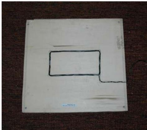
**Figure 5.19: Simulated long-loop for analysis of queue detectors**
