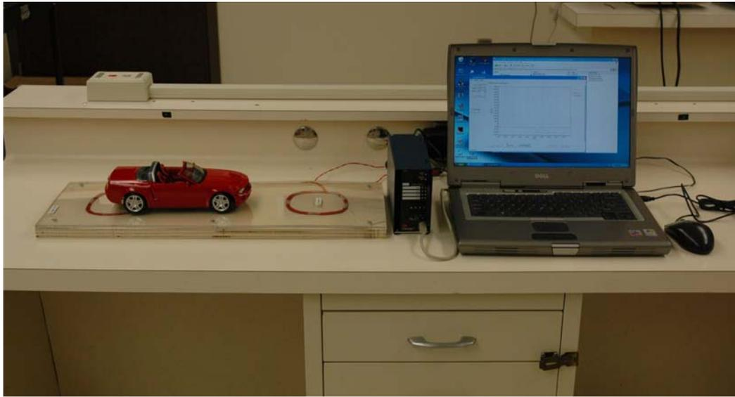
**Figure 5.18: Hardware-in-Loop test system for inductance signature analysis**
