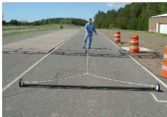
**Figure 5.3: Apparatus used for loop system impulse response**
