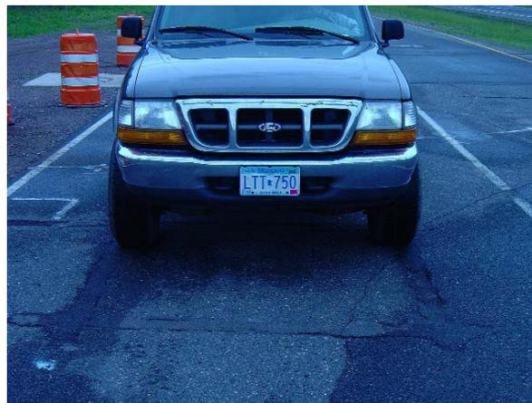
**Figure 5.4: Ford Ranger used to collect inductance waveforms at various speeds**
