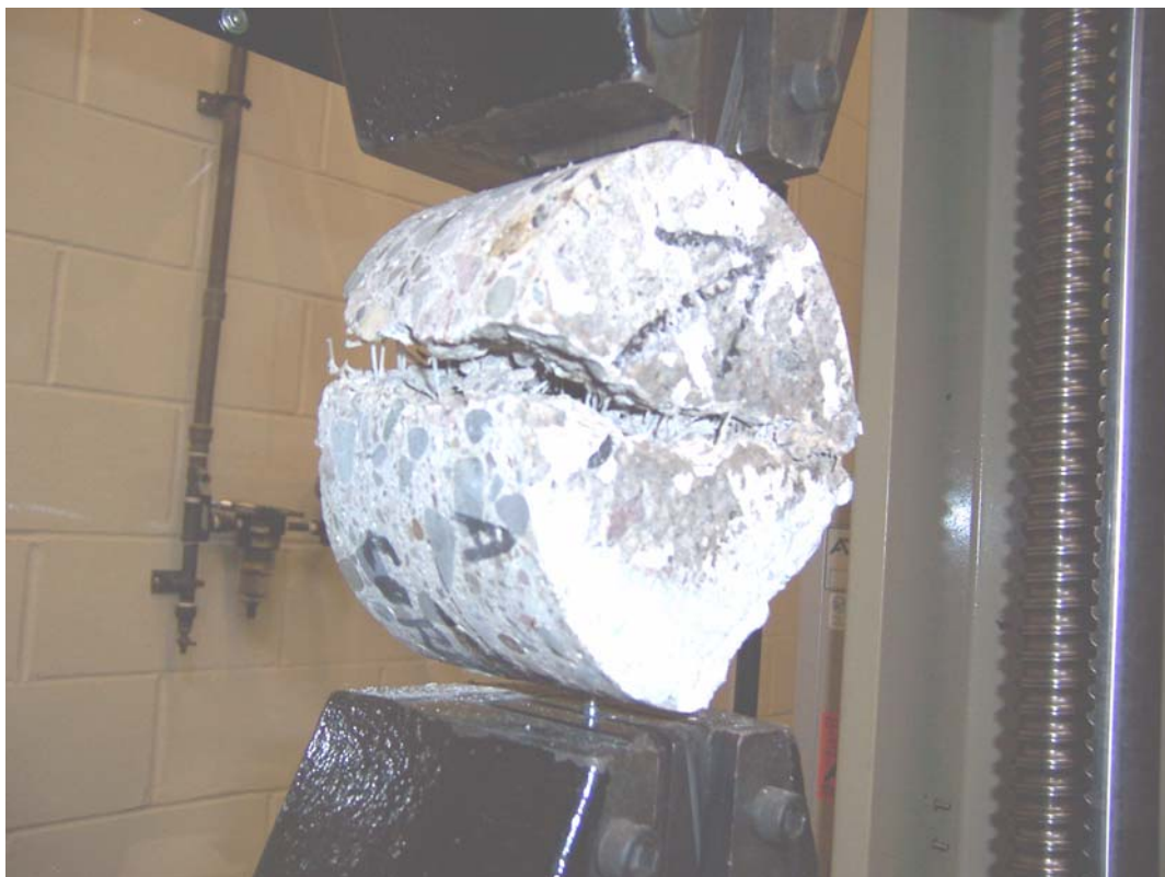
Photo 3.5. Core sample during testing. Note fibers spanning crack.
