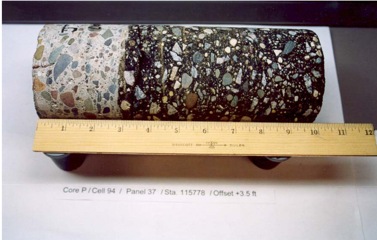
Photo 3.14 Core sample “I” showing top-down partial depth cracking.
