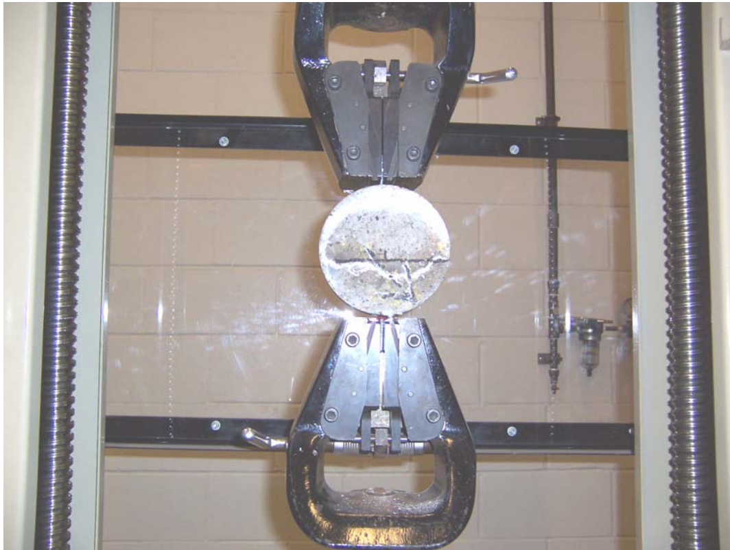
Photo 3.5. Core sample during testing. Note fibers spanning crack.
