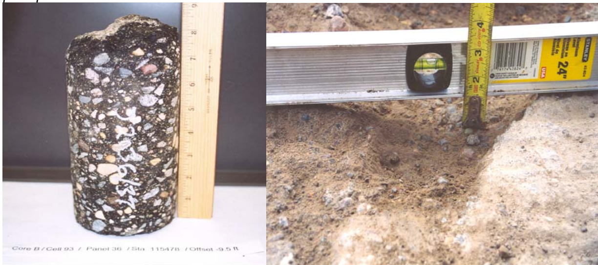
Photo 3.16 Core sample “B” and close-up of forensic area “A” showing deformation in HMA from punchout in UTW.
