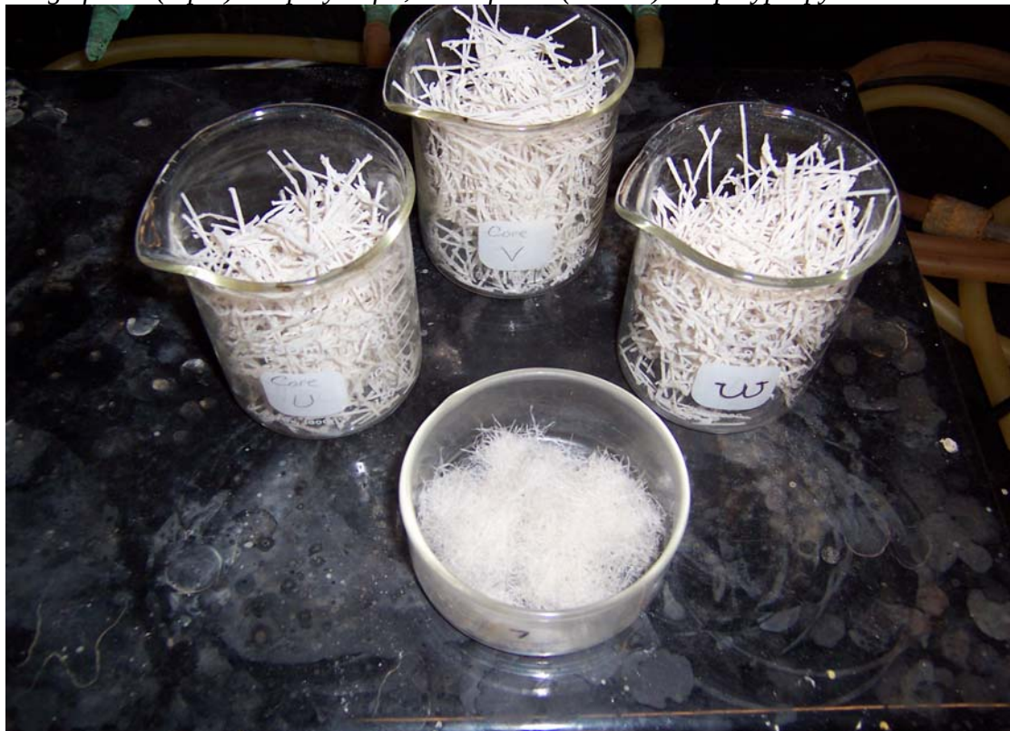
Photo 3.8 Fibers removed from core samples. Large fibers (top 3) are polyolefin, small fibers (bottom) are polypropylene.
