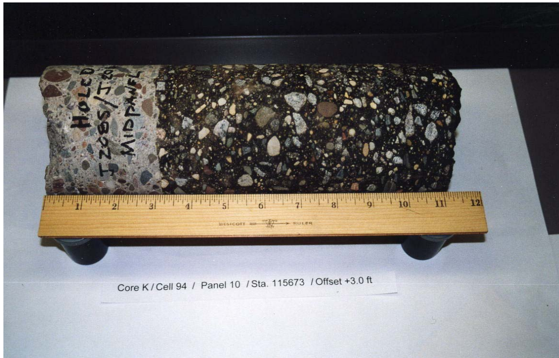
Photo 3.1. Core sample showing bonded layers of HMA and UTW.
