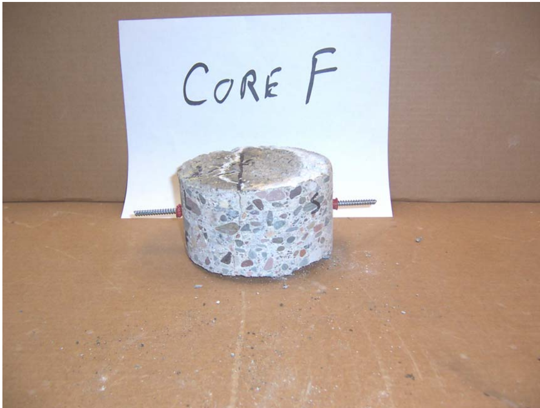
Photo 3.3. Steel anchor screws installed into core before testing.
