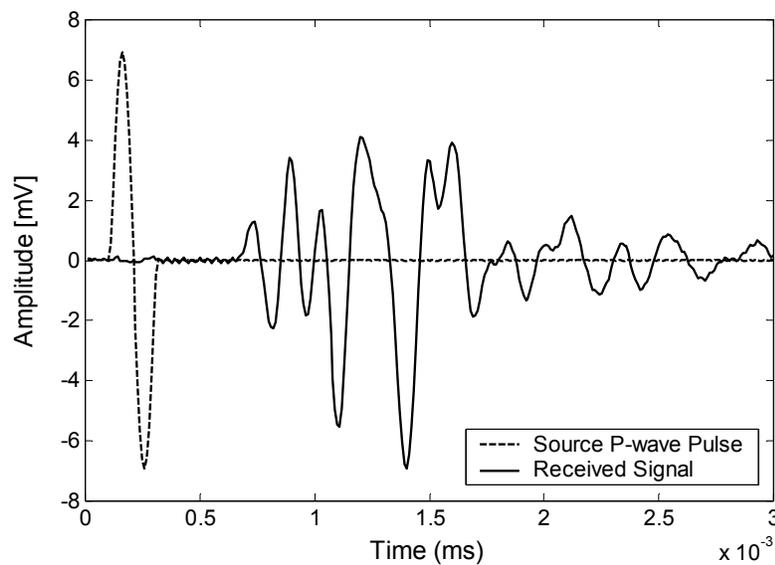
Figure 3.19: P-Wave Source and Receiver Time Histories
