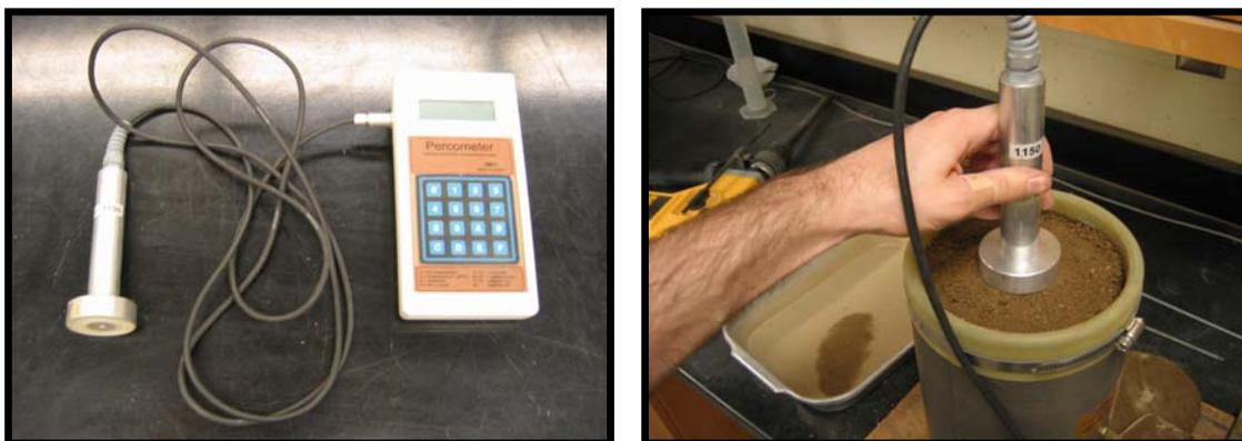
Figure 3.13: Percometer Measurement
