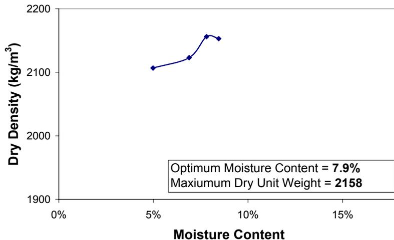
Figure 3.11: Compaction Data for Sample A
