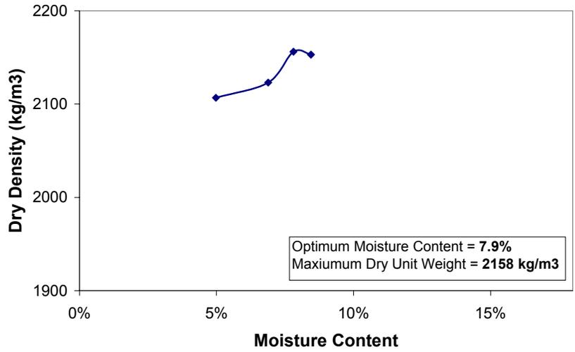
Figure A.2: Standard Proctor Compaction Curve for Sample A
