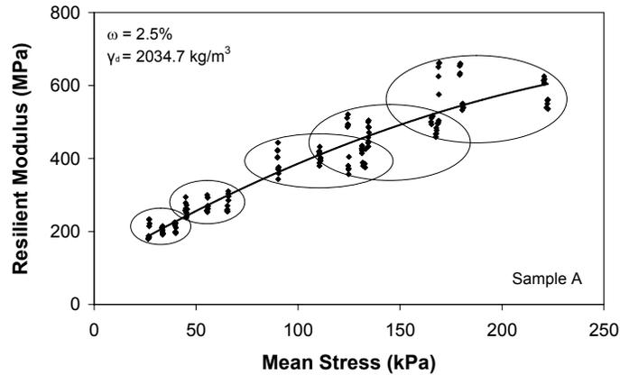
Figure 4.8:  $M_R$  Versus Mean Stress for Sample A
