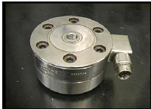
Figure 3.4: Load Cell
