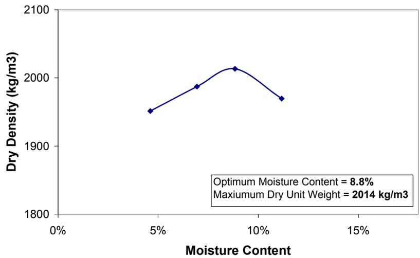
Figure A.7: Standard Proctor Compaction Curve for Sample N
