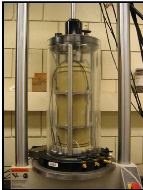
Figure 3.2: Triaxial Cell Containing Specimen
