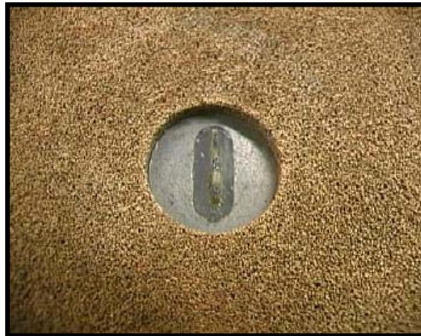
Figure 3.6: Bender Element Cantilever Strip
