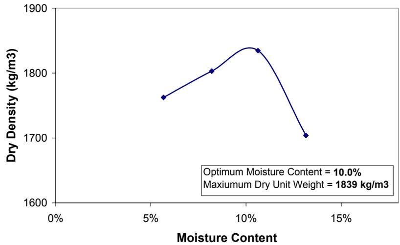
Figure A.3: Standard Proctor Compaction Curve for Sample D
