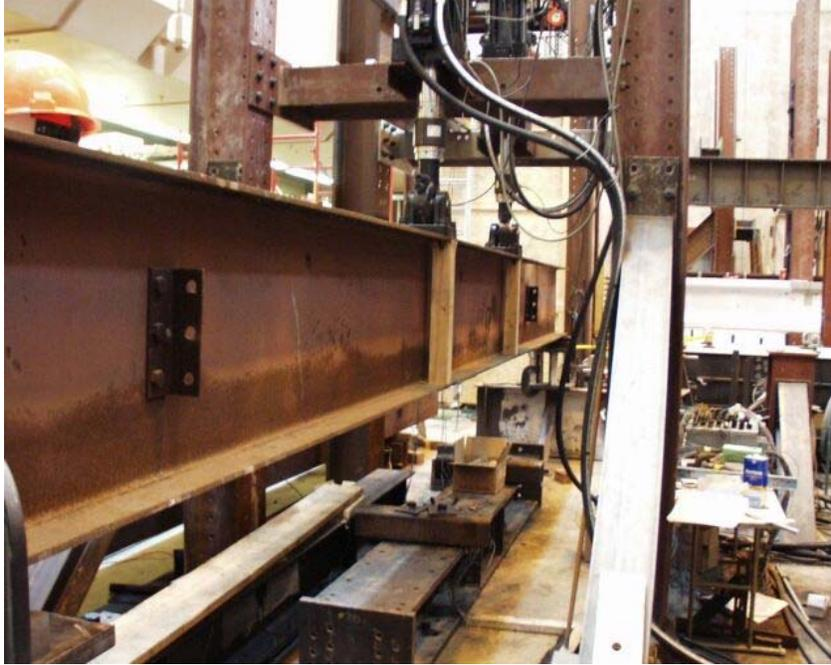
**Figure 4.35 Test Setup for Cyclic Loading Tests on W27x84**
