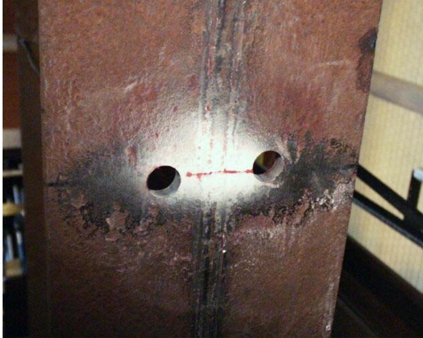
**Figure 4.43 Specimen with Crack and Holes (R-3-1)**
