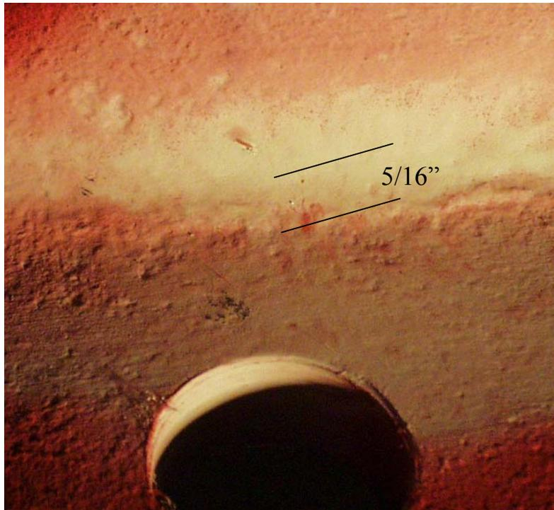
Figure 4.39 Crack Reached Inner Surface of Tension Flange
