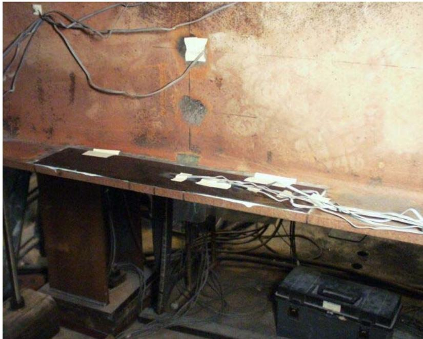
**Figure 4.44 Rehabilitated Specimen with Bonded CFRP Strip**
