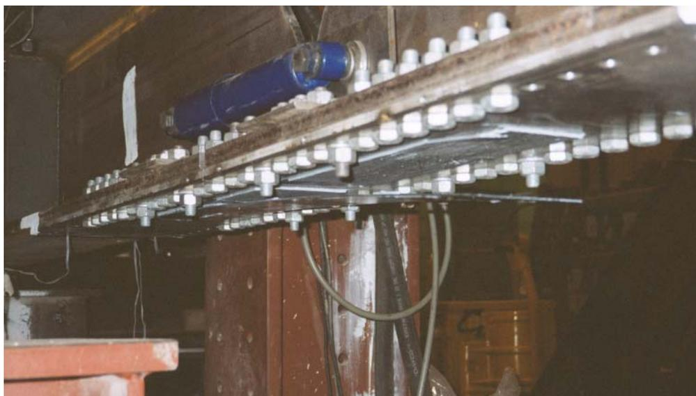
**Figure 4.1 Post Failure Photograph - Specimen 1-3**
