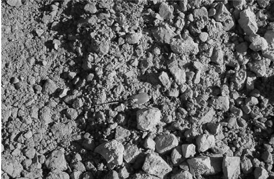
**Figure 3.4. 6-in. (300-mm) Breaker Run Limestone.**
