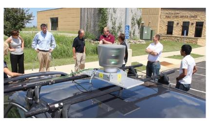
TAP members attend a demonstration of light detection and ranging (lidar) technology, which can capture 3-D images for analyzing traffic, tracking assets and more.
