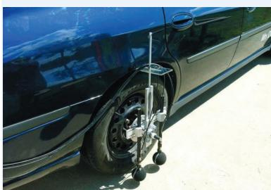
To measure noise from tire-pavement interaction, researchers used onboard sound intensity testing in which microphones are mounted near the interface of tire and pavement.
