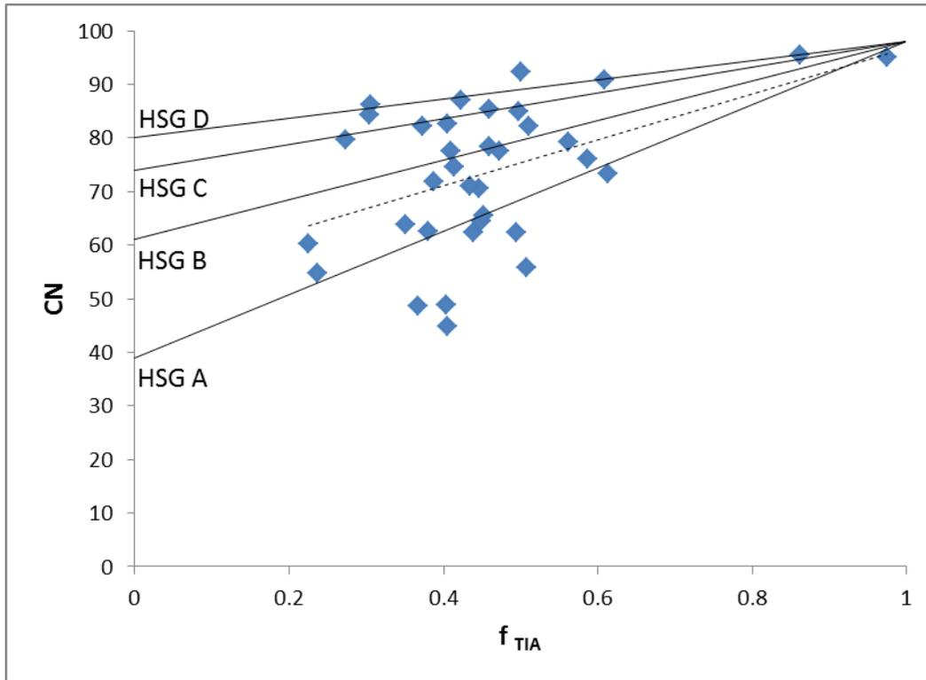
**Figure 5.11 Comparison of the regression line for actual CN vs. TIA fraction (dashed line) with the TR-55 CN trends in different hydrologic soil groups (solid lines). The data points are as in Figure 5.10.**
