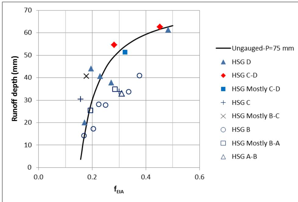
**Figure 5.17 Using hydrologic soil group (HSG) to partially explain the scatter of the actual data in comparison to the developed Runoff depth vs. EIA fraction curve for ungauged watersheds with P=75 mm.**
