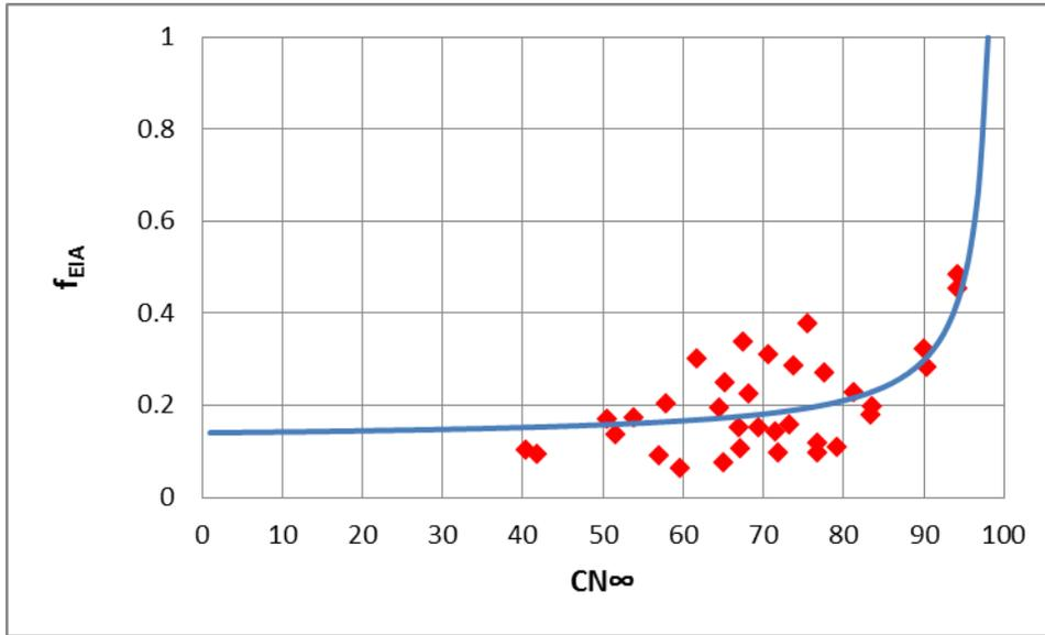
**Figure C.2 Comparison of the actual  $f_{EIA}$  and  $CN_{\infty}$  values in gauged watersheds with the presented curve for ungauged watersheds in the case of  $\lambda=0.05$ . The actual  $f_{EIA}$  values have been estimated based on the proposed SWLS method and the actual  $CN_{\infty}$  values have been calculated using the Hawkins' asymptotic CN method (Hawkins 1993) and the assumption of  $I_a = 0.05S$ .**
