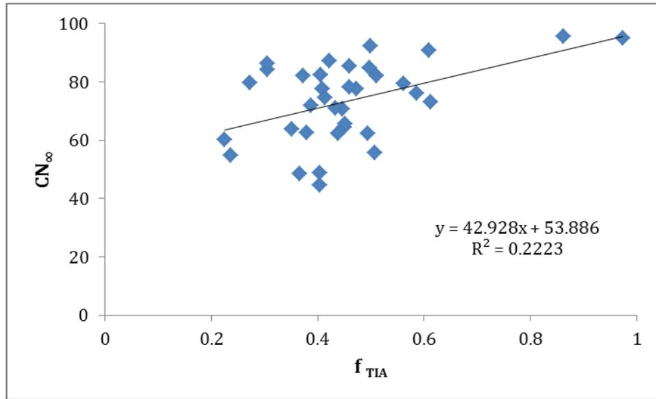
**Figure 5.10** Plot of actual CN versus TA fraction in the watersheds of study. Although the  $R^2$  does not show a strong correlation, it can be explained by the narrow range of  $CN_{\infty}$  values and the regression equation is in a good agreement with the TR-55 CN table in extreme conditions of  $f_{TIA}=0$  and 1.
