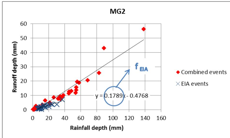
**Figure 3.2 Application of the method of Boyd et al. (1993) to the MG2 watershed in Maple Grove, MN. 17.9% of the entire MG2 watershed is hydraulically connected to the drainage system based on this method.**
