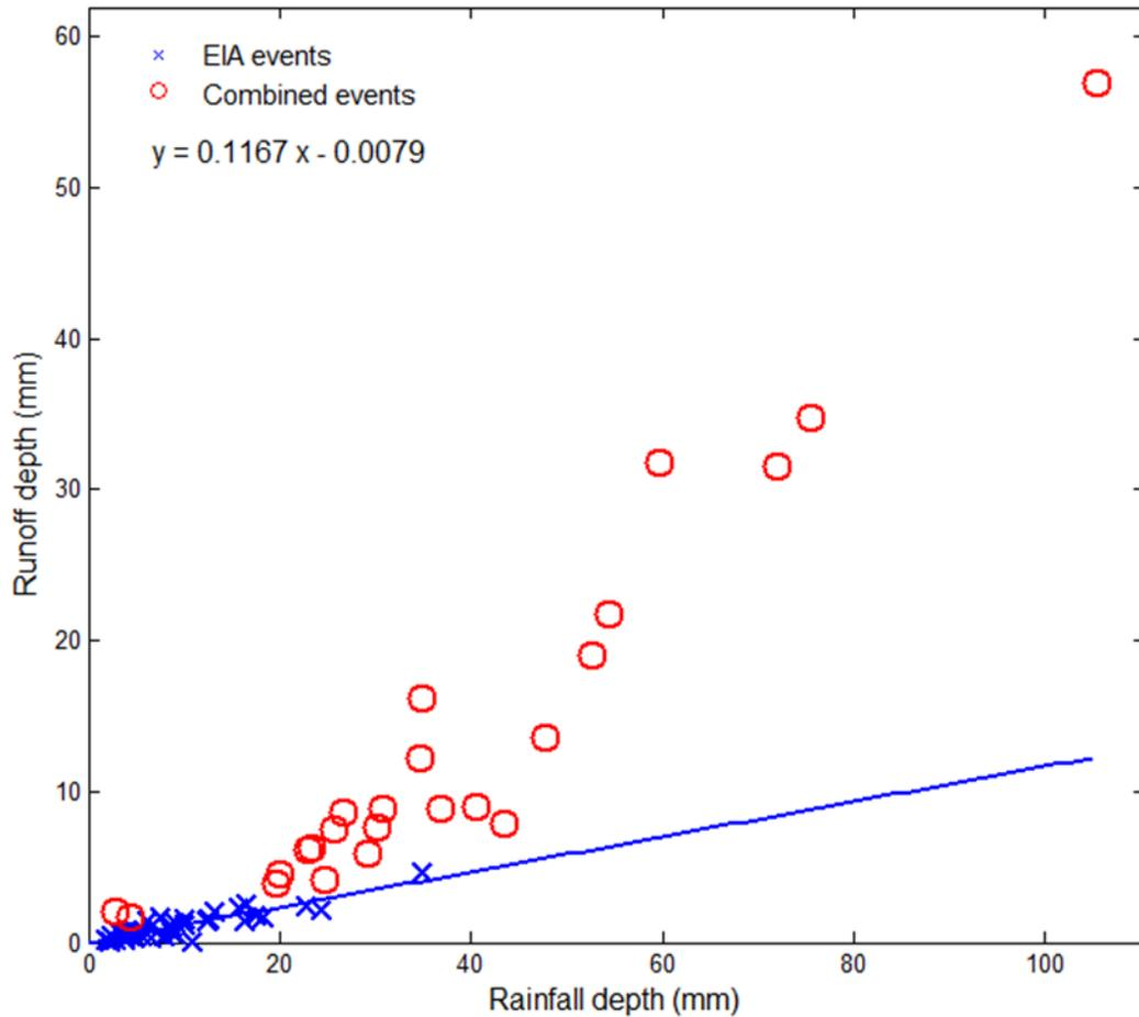
**Figure 3.6 Application of the SWLS ( $\max(2 \textit{pseudo SE}_{WLS}, 1\textit{mm})$ ) method to the MG1 catchment in Maple Grove, MN. The estimated EIA fraction has decreased to 0.117 and less small rainfalls have been categorized as combined events in the SWLS ( $\max(2 \textit{pseudo SE}_{WLS}, 1\textit{mm})$ ) method. The SWLS method leads to the minimum variance (uncertainty) in the estimated EIA fraction.**
