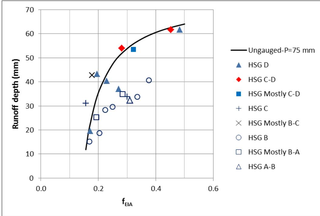
**Figure C.7 Using hydrologic soil group (HSG) to partially explain the scatter of the actual data in comparison to the developed Runoff depth vs. EIA fraction curve for ungauged watersheds with  $P=75$  mm in the case  $\lambda=0.05$ .**
