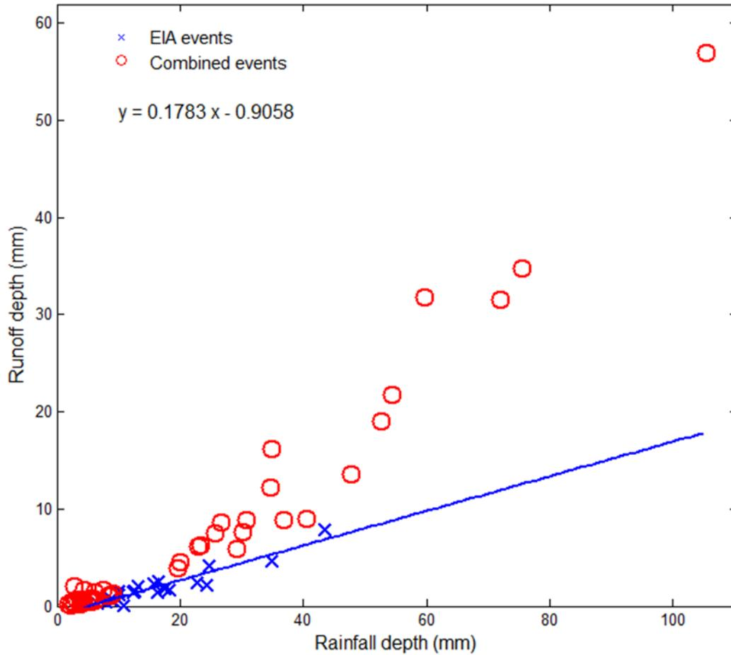
**Figure 3.5 Application of the SOLS (1 mm) method to the MG1 catchment in Maple Grove, MN. The graph shows that 17.8% of the entire MG1 area is hydraulically connected to the drainage system based on the SOLS (1 mm) method.**
