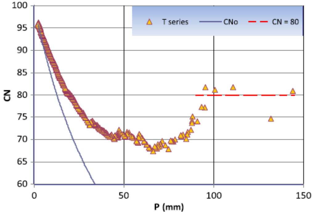
**Figure 5.4 Example of the violent behavior in Delia watershed at Pozzillo station in Sicily, Italy (from D’Asaro and Grillone, 2012).  $CN_0$  is the CN at which runoff starts and  $CN_\infty$  is determined as 80 in this watershed.**
