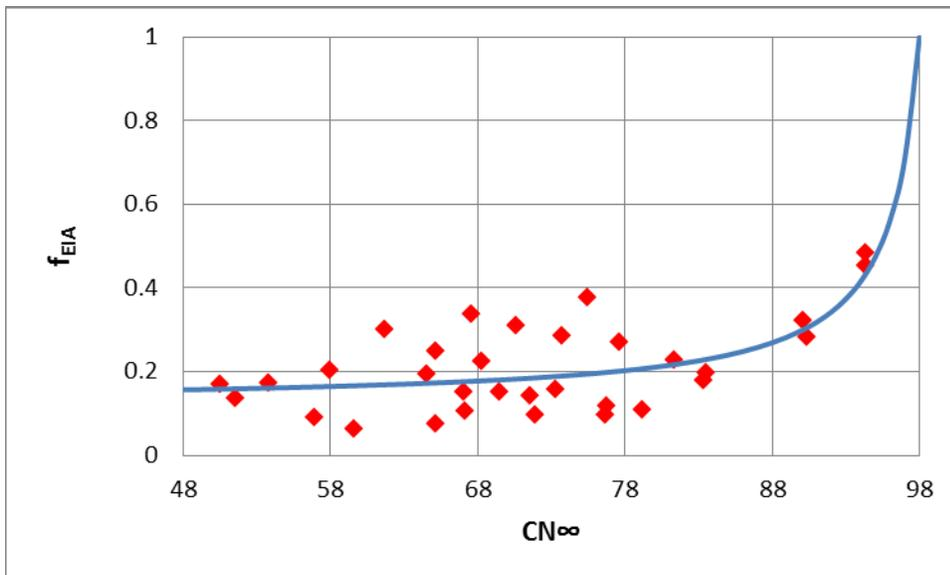
**Figure C.3 Comparison of the actual  $f_{EIA}$  and  $CN_{\infty}$  values in gauged watersheds with the presented curve for ungauged watersheds in the case of  $\lambda=0.05$ .  $CN_{\infty}$  values are limited to the range of 48 and 98 based on the condition of  $0.4 \leq \alpha \leq 1$ .**
