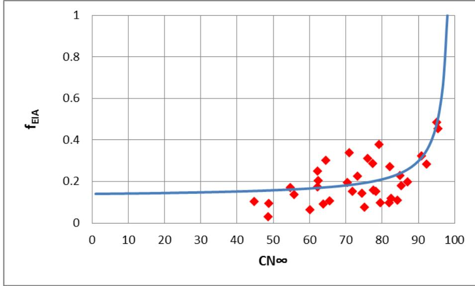
**Figure 5.8 Comparison of the actual  $f_{EIA}$  and  $CN_{\infty}$  values in gauged watersheds with the presented curve for ungauged watersheds. The actual  $f_{EIA}$  values have been estimated based on the proposed SWLS method and the  $CN_{\infty}$  values have been calculated using the Hawkins' CN method (Hawkins 1993).**
