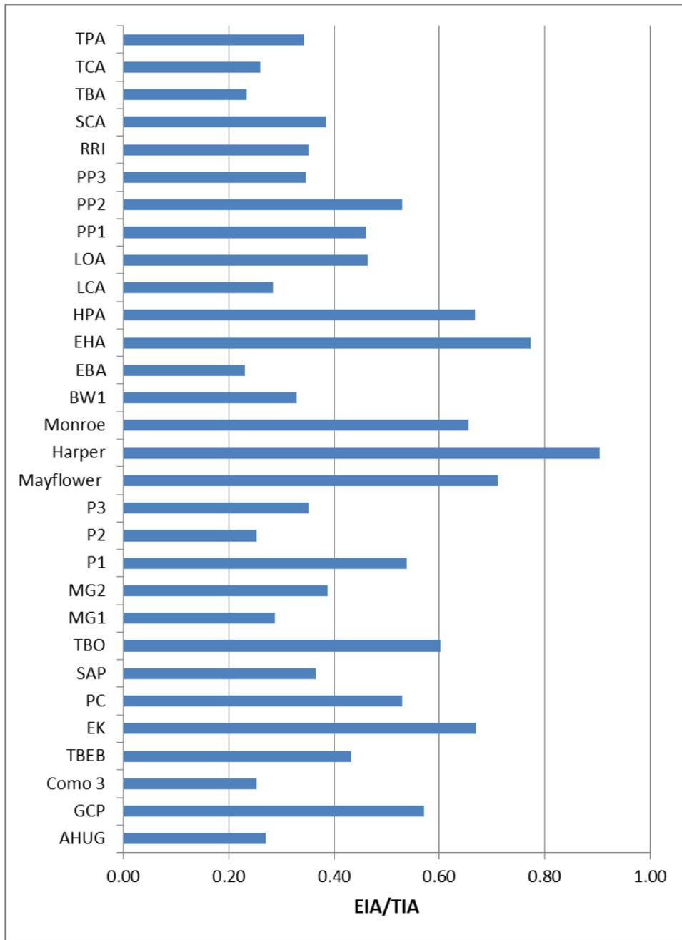
**Figure 4.6 The ratio of EIA/TIA for all the study sites with residential land uses (30 sites). The chart shows that only about half of the impervious surfaces are hydraulically connected to the drainage system.**
