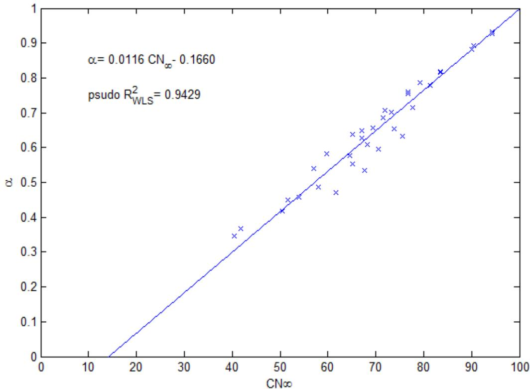
**Figure C.1** Plot of  $\alpha$  versus  $CN_{\infty}$  for the case of  $\lambda=0.05$ . Since  $\alpha$  is the ratio of  $CN_r/98$ , the regression shows a strong correlation between  $CN_r$  and  $CN_{\infty}$  in the watersheds of study.
