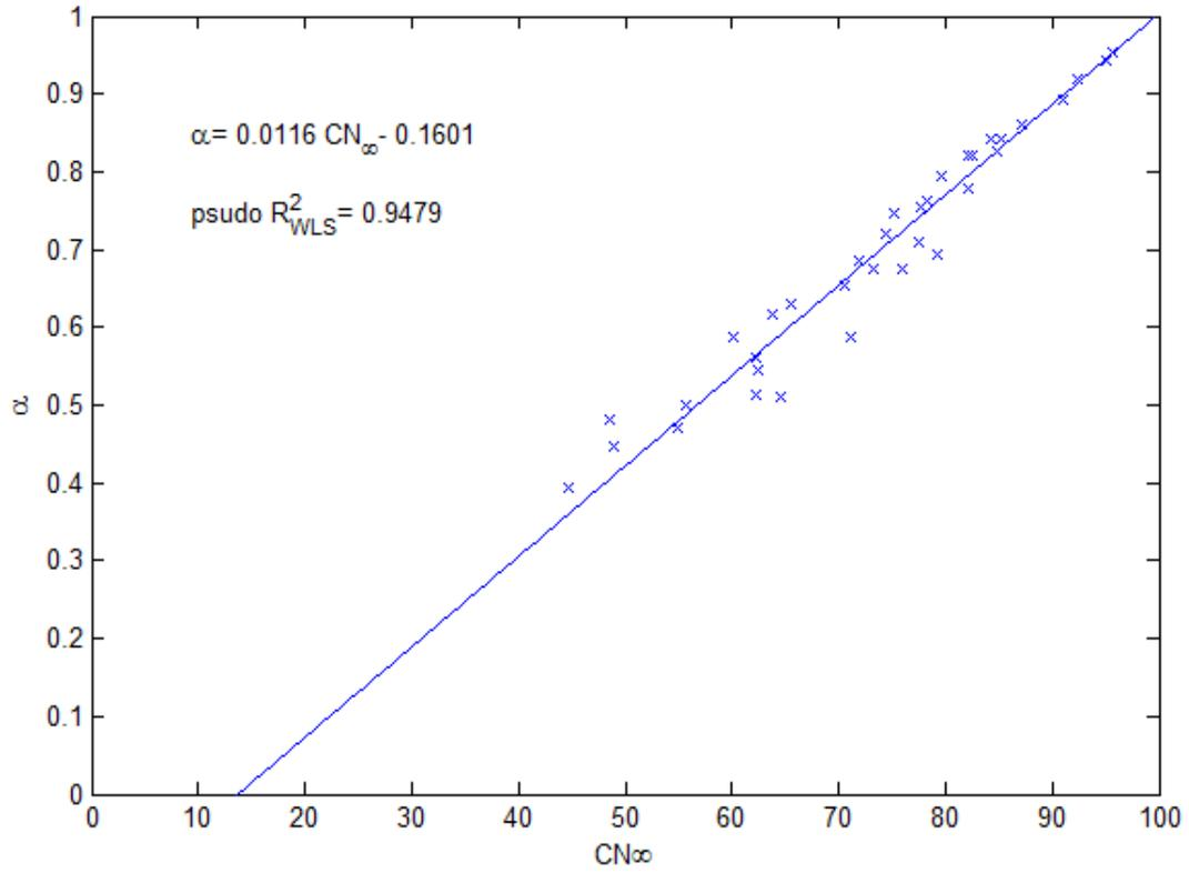
**Figure 5.6 Plot of  $\alpha$  versus  $CN_{\infty}$ . Since  $\alpha$  is the ratio of  $CN_r/98$ , the regression shows a strong correlation between  $CN_r$  and  $CN_{\infty}$  in the watersheds of study.**
