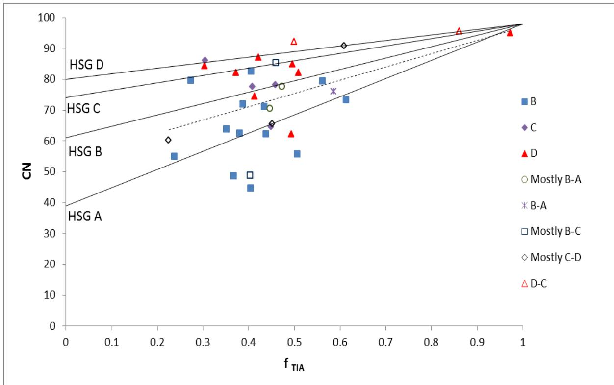
**Figure 5.13 Comparison of the TR-55 CN trends in different hydrologic soil groups (solid lines) with the actual HSGs from SSURGO dataset. The data points are the same as Figure 5.13 and the dashed line is the regression line for actual CN vs. TA fraction. The scatter of the data around corresponding lines especially for lower  $f_{TIA}$  values indicates the inaccuracies of representing the actual CN values in a watershed with different HSGs and TR-55 CN values.**
