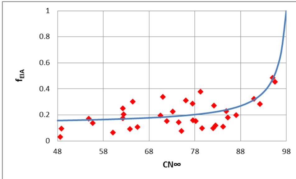
**Figure 5.9 Comparison of the actual  $f_{EIA}$  and  $CN_{\infty}$  values in gauged watersheds with the presented curve for ungauged watersheds.  $CN_{\infty}$  values are limited to the range of 48 and 98 based on the condition of  $0.4 \leq \alpha \leq 1$ .**
