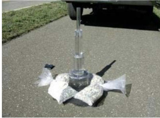
**Figure 2.27 Cascaded Field Permeameter'**
