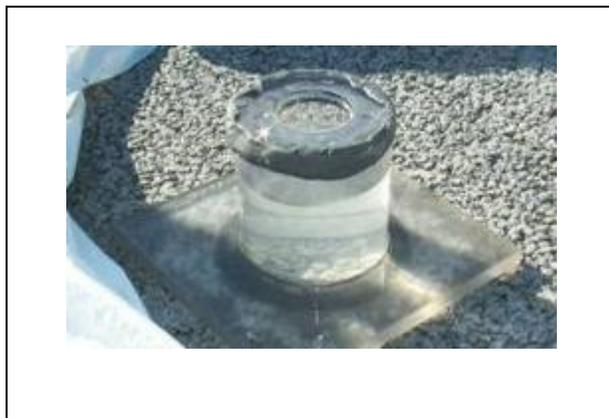
**Figure 3. 30 Field Permeameter**
