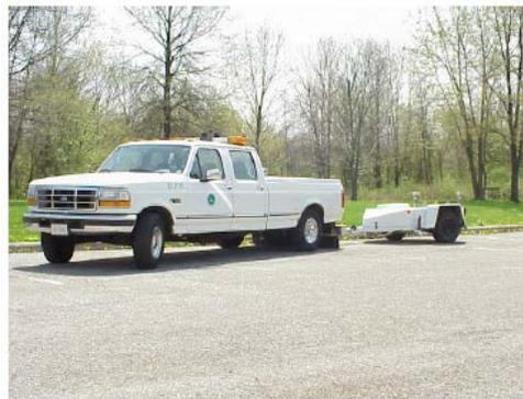
**Figure 1.4-Locked Wheel Skid Trailer [23]**
