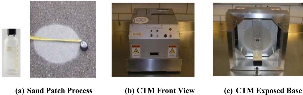
**Figure 1.6 Measurement of Texture Depth [23]**
