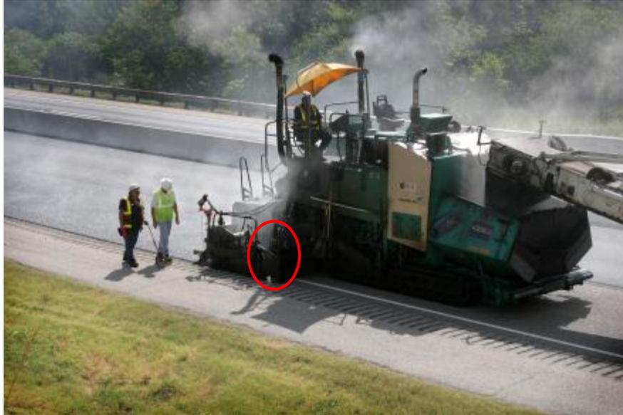
**Figure 2.6: Nova Chip Paver**
