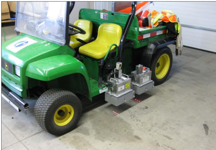
**Figure 1.8: Lightweight Inertial Surface Analyzer (LISA) [15]**
