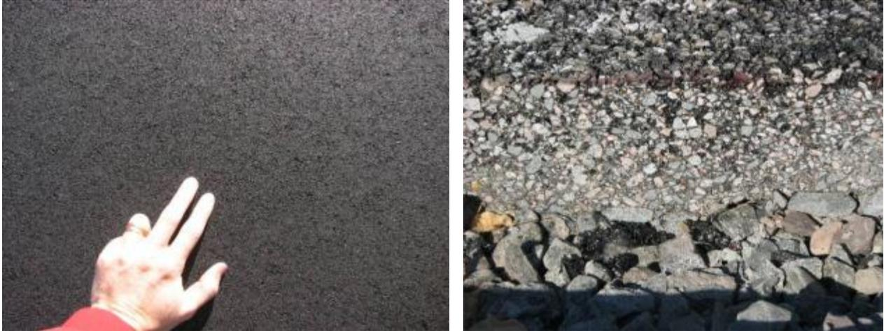
**Figure 3.4 4.75 Taconite [Left] and Cross-Section of Porous HMA [Right]**
