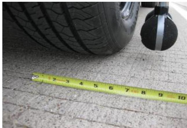
**Figure 2.23 On Board Sound Intensity Test Setup and Microphone Close Up View**
