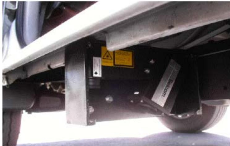
**Figure 1.13: FDOT Unit High-Speed Laser System [21].**
