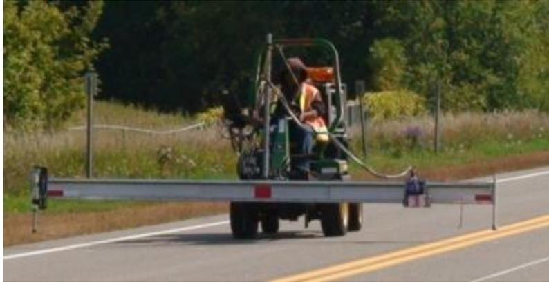
**Figure 3.34 Automated Laser Profile System (ALPS)**
