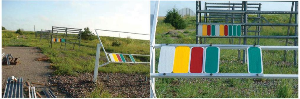
The test deck installed at MnROAD includes color and sheeting material combinations and will ultimately provide accurate data about how long it will take for a sign’s retroreflectivity to drop below MUTCD standards.
