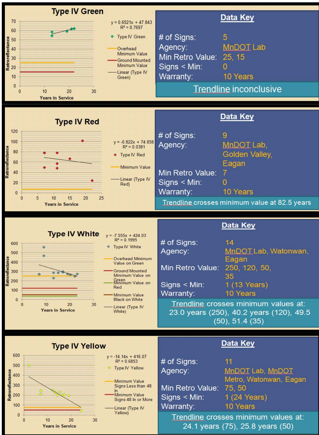
Figure 3.3 – Type IV Sheeting Retroreflectivity Results
