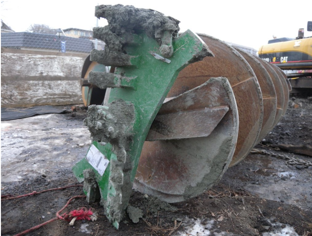
Figure 7.4 Cutter Head and Augers used for Auger Boring (CNA Consulting Engineers)
