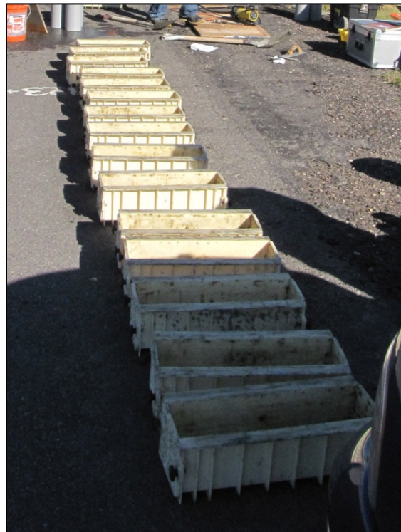
Figure 8: Set of 15 beam molds for maturity curve development.
