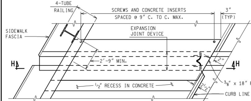
PLAN AT 4 TUBE (PEDESTRIAN) STEEL RAILING
