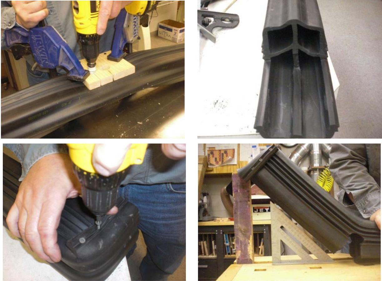
**Figure 29: A curb kick-up procedure for the JP compression seal.**
