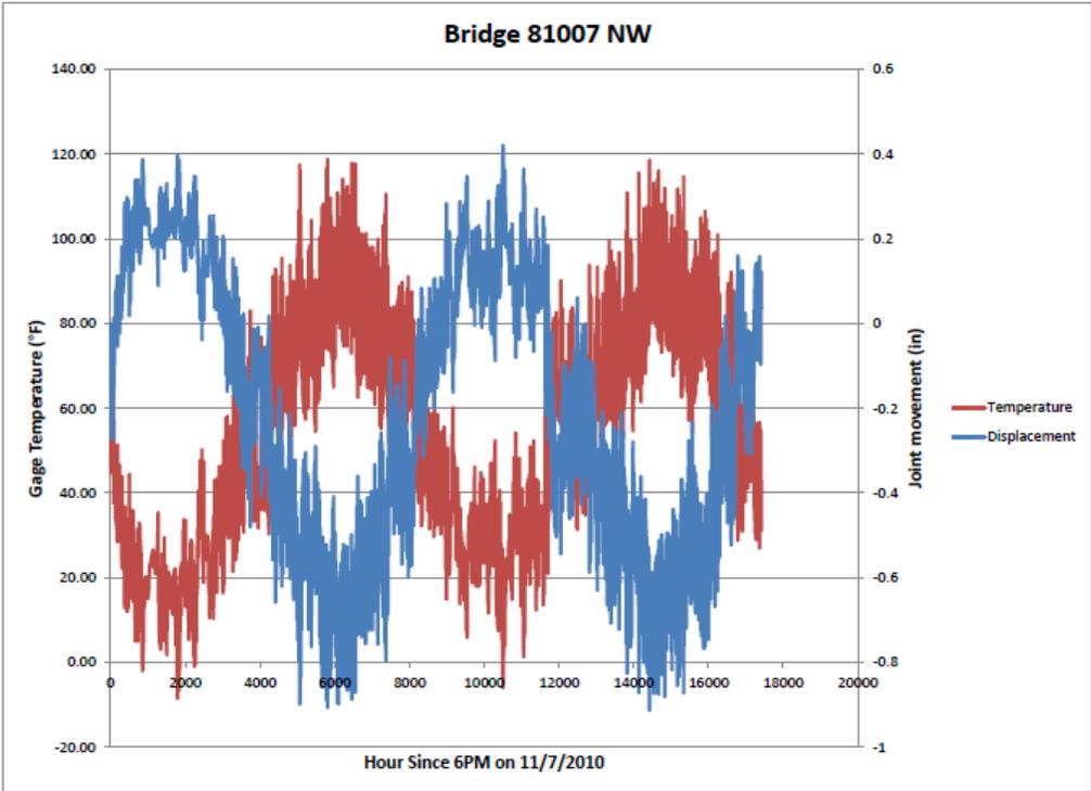
Figure 17: Bridge 81007NW displacement and temperature versus time.
