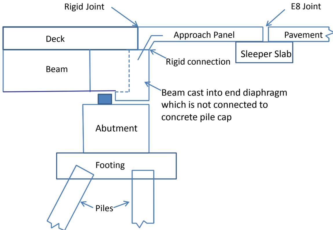
**Figure 3: Schematic details of a semi-integral abutment.**
