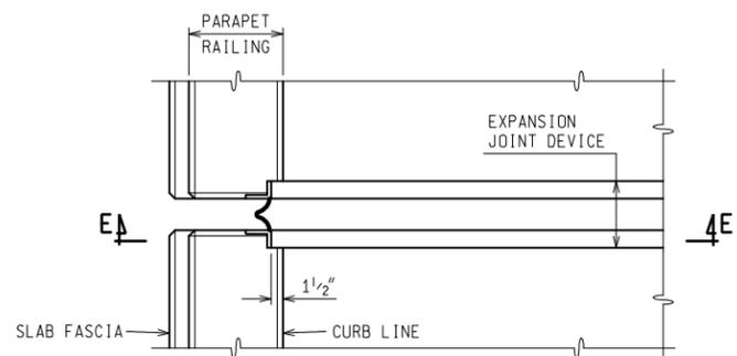
PLAN AT FLUSH MOUNT PARAPET RAILING
