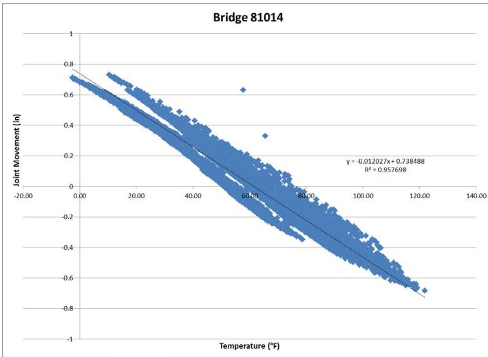
**Figure 24: Bridge 81014 movement versus temperature.**
