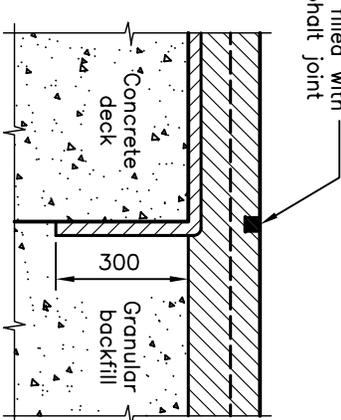
**JOINT BETWEEN CONCRETE DECK AND GRANULAR BACKFILL**
