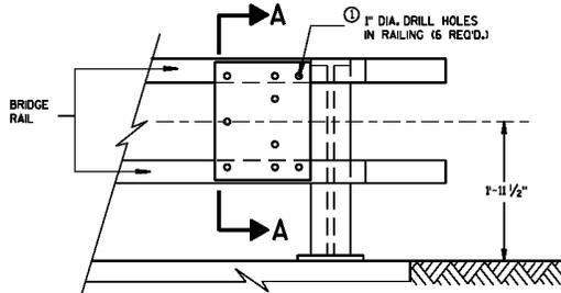
**BACK-UP PLATE MOUNTING ONTO BRIDGE RAILING**
