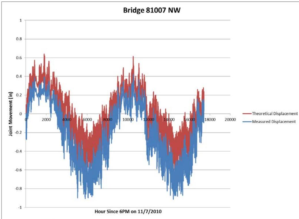
**Figure 25: Theoretical and measured displacement versus time.**
