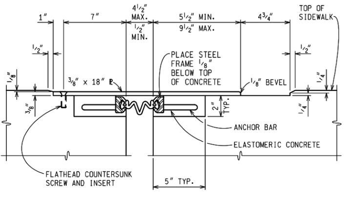
SECTION THROUGH EXPANSION JOINT AND COVER PLATE
