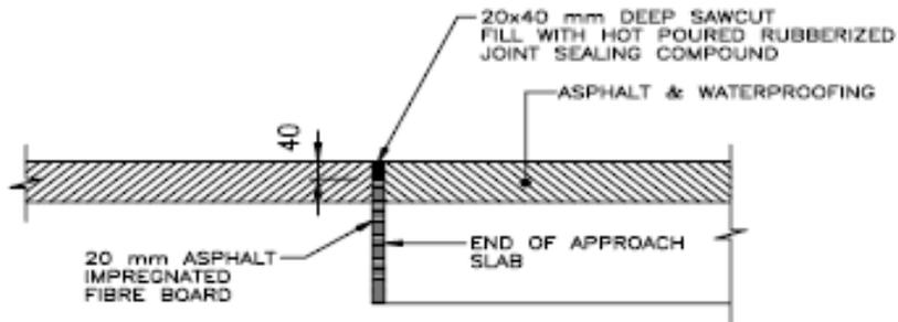
2. For integral and semi integral bridges where the expected movement at the end of the approach slab is between 25 and 50 mm, the requirements shall be as shown below:
