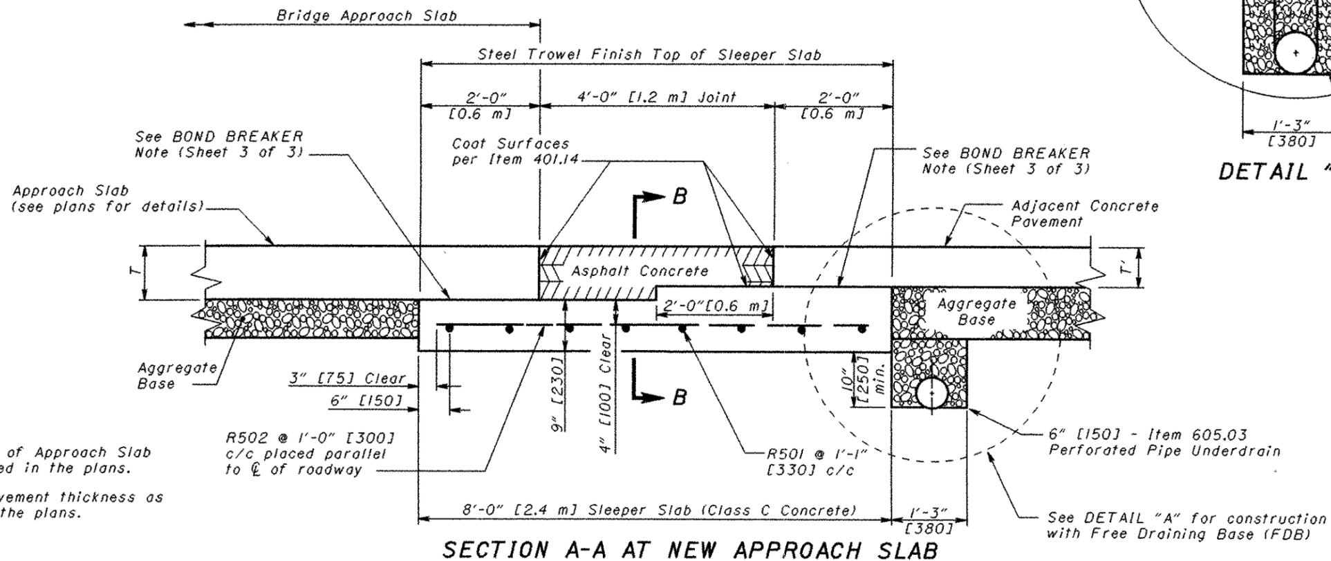
**SECTION A-A AT NEW APPROACH SLAB**
