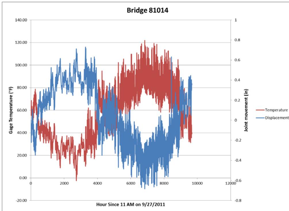
**Figure 20: Bridge 81014 displacement and temperature versus time.**
