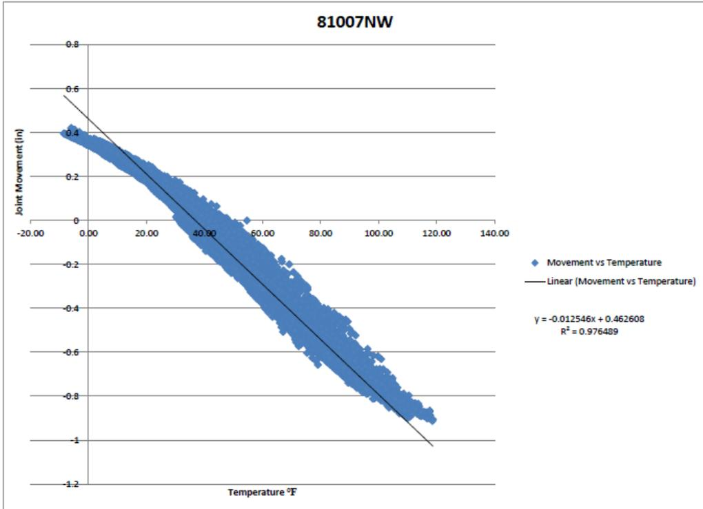
**Figure 21: Bridge 81007NW movement versus temperature.**
