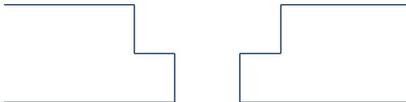
**Figure 7: Example of a concrete blockout shape.**
