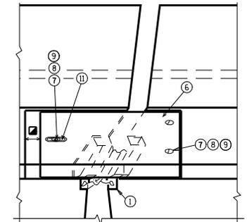
**VIEW OF PARAPET PLATES FROM ROADWAY**
