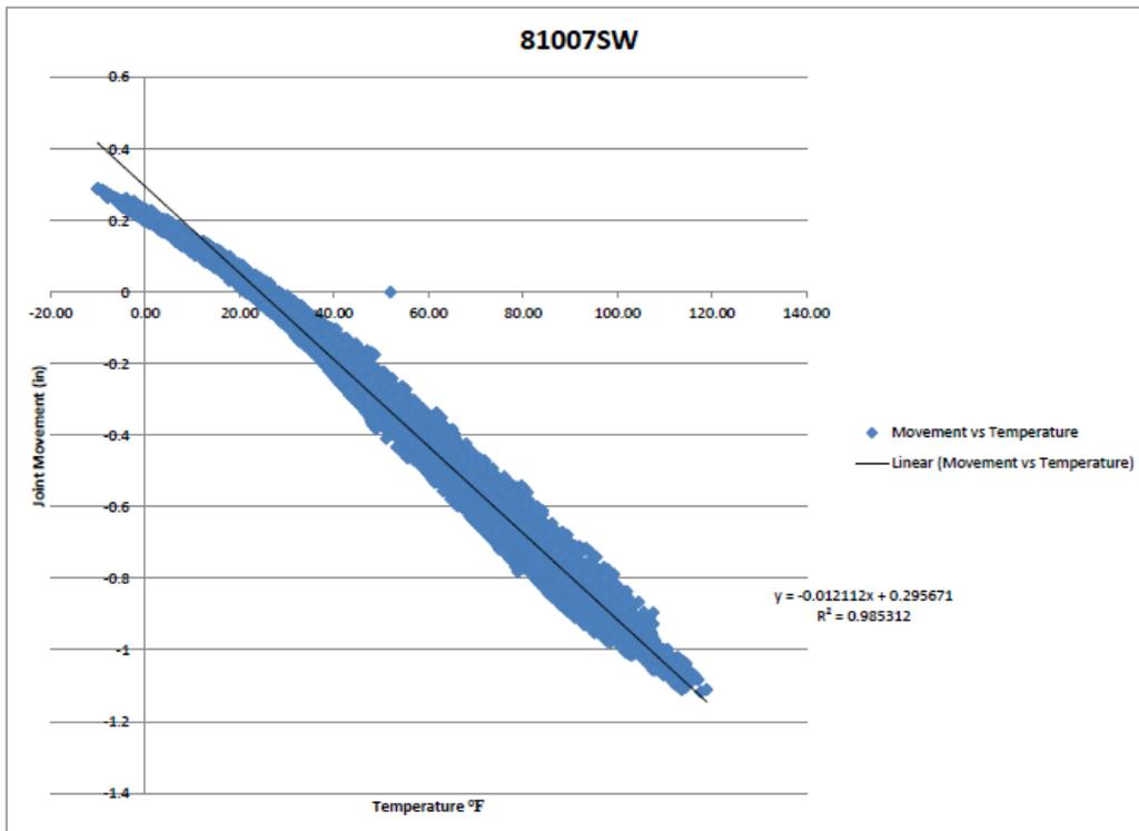
**Figure 22: Bridge 81007SW movement versus temperature.**
