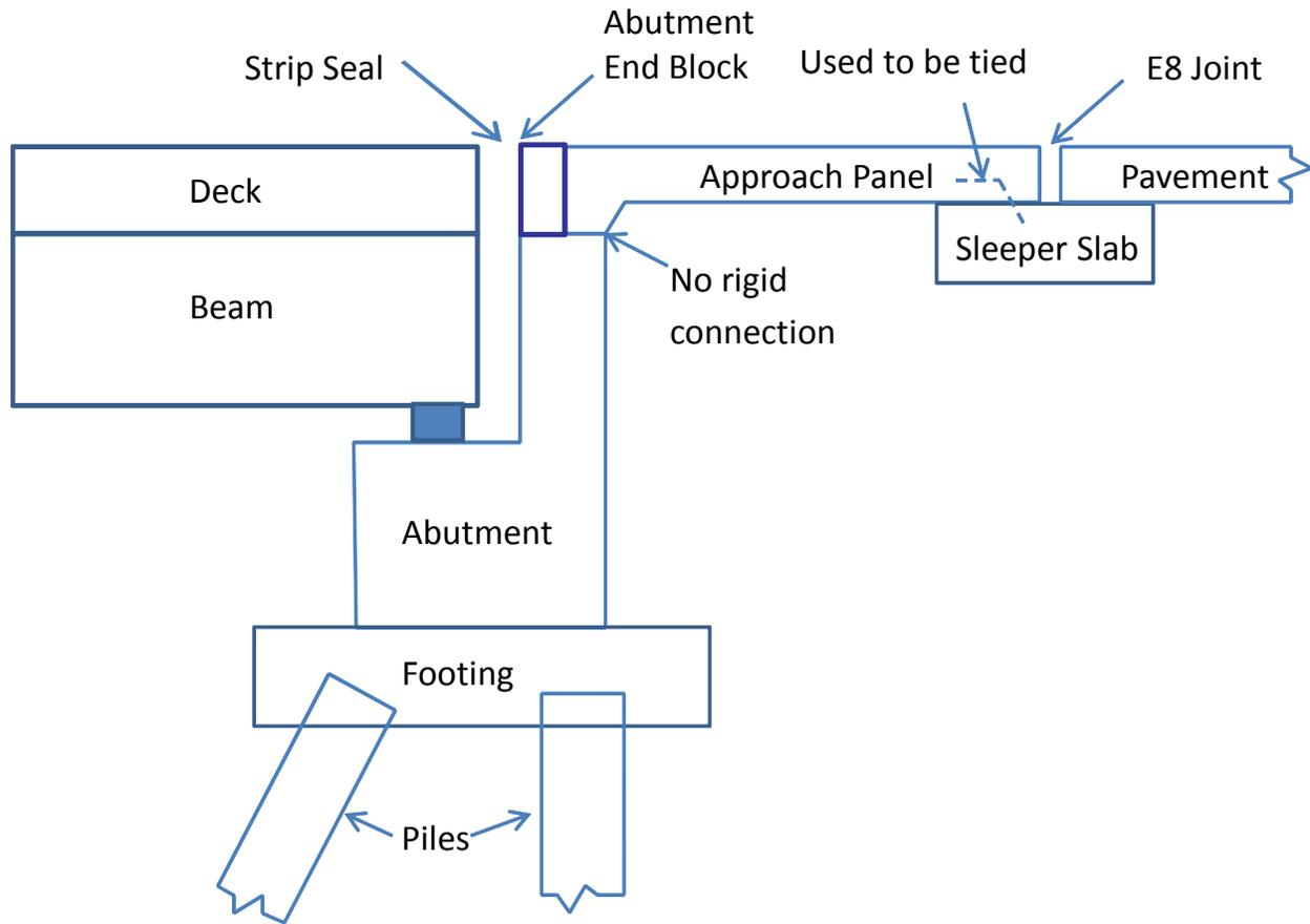
**Figure 1: Schematic details of a parapet-type abutment.**
