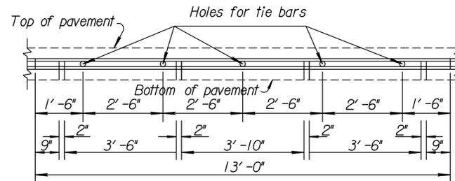
To be used only against forms. Shall not extend through contraction joints.
