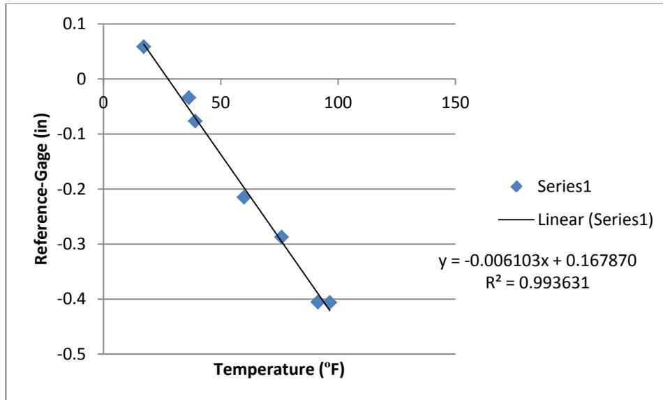
**Figure 16: Adjustment factor to reconcile reference readings with gage readings for Bridge 81007NW.**
