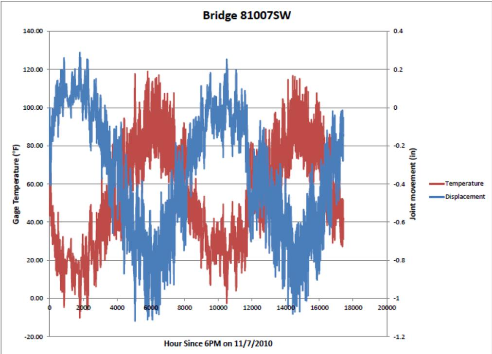
Figure 18: Bridge 81007SW displacement and temperature versus time.
