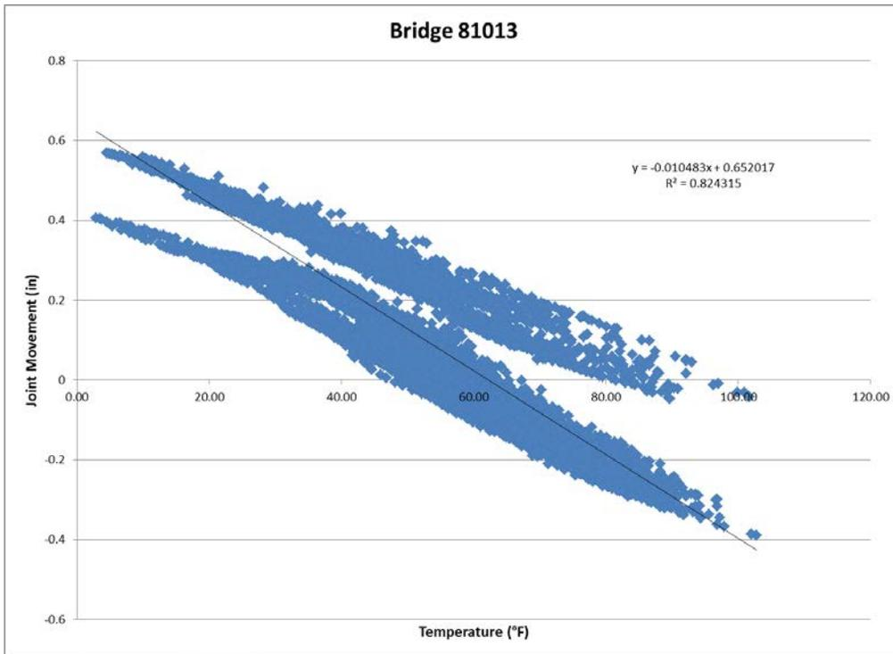
**Figure 23: Bridge 81013 movement versus temperature.**
