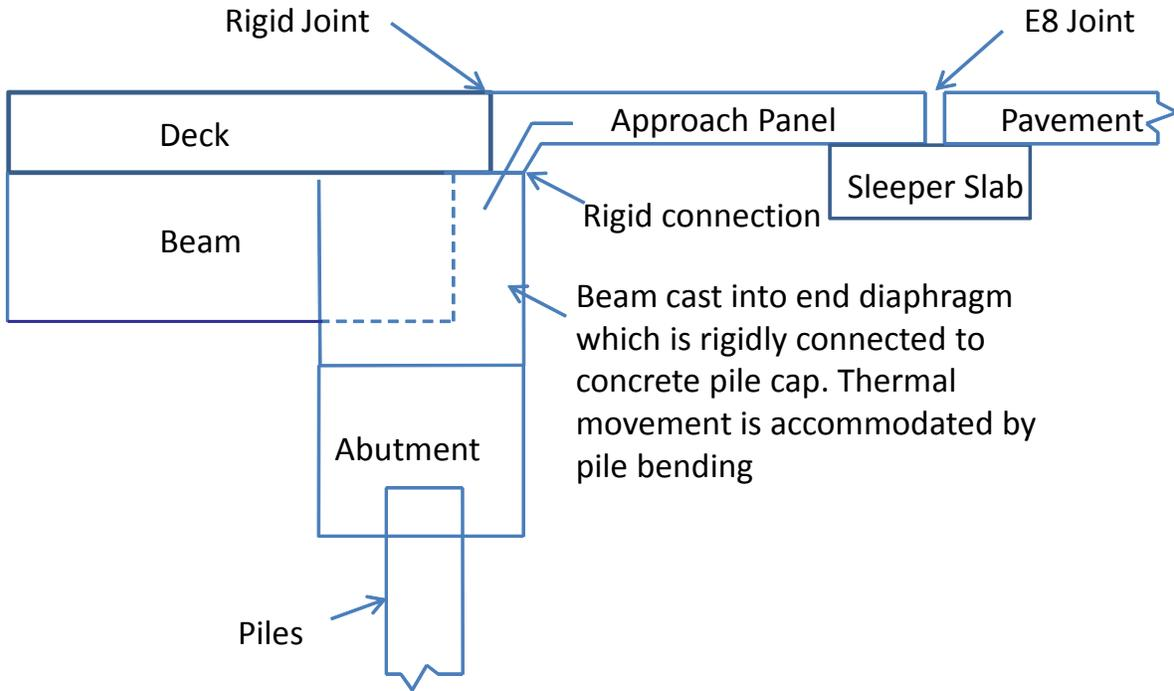
**Figure 2: Schematic details of an integral abutment.**
