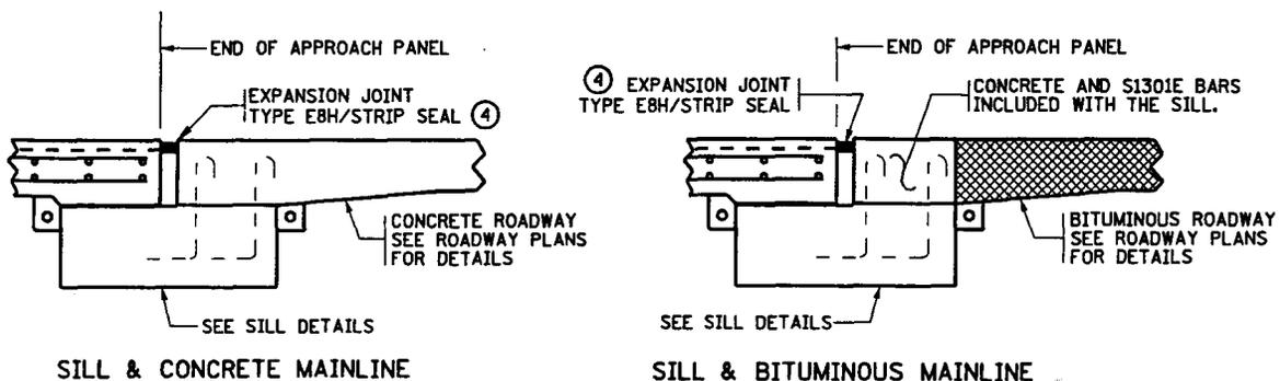
Figure 5: Approach slab to roadway connection details.
