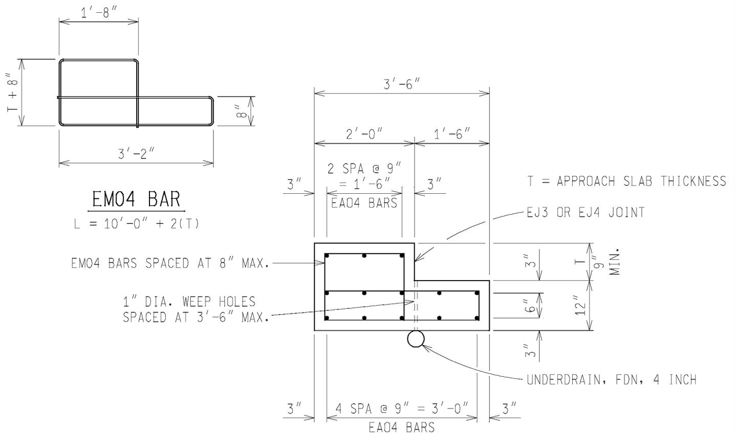
**TYPICAL SECTION THRU SLEEPER SLAB WITH HMA APPROACH**
