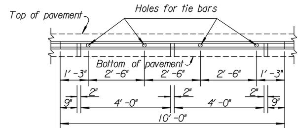
To be used only against forms. Shall not extend through contraction joints.
