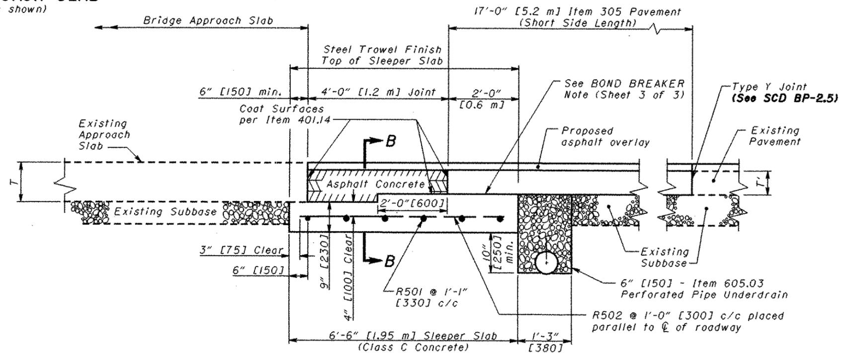
**SECTION A-A AT EXISTING APPROACH SLAB**
