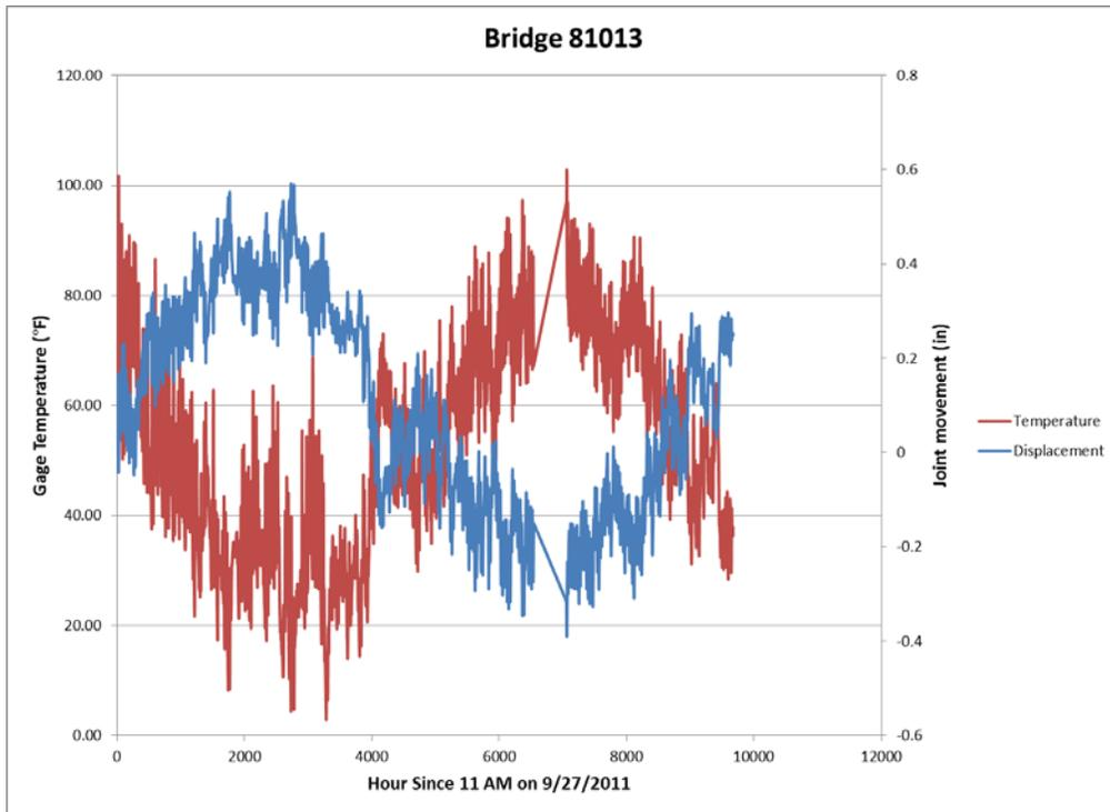
**Figure 19: Bridge 81013 displacement and temperature versus time.**
