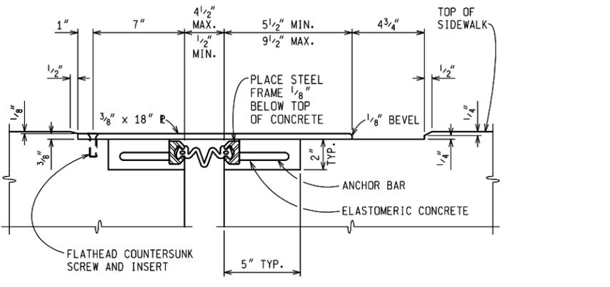
SECTION THROUGH EXPANSION JOINT AND COVER PLATE
