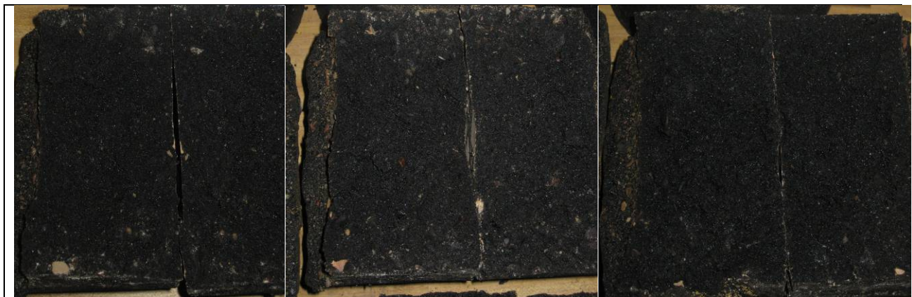
Figure 2.11. Visual Examination of APA ‘wet’ specimens
