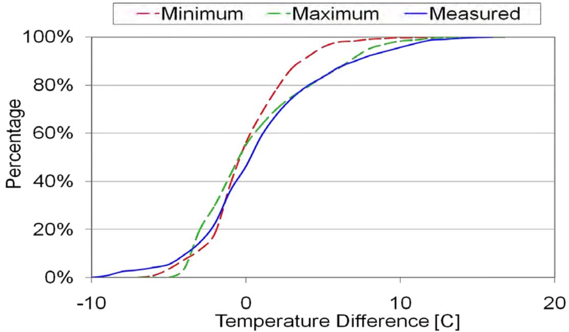
**Figure 2-27: Measured versus modeled cumulative frequency distribution for thermal gradient through JPCP pavement in March with  $k = 1.25 \text{ BTU / hr-ft-}^\circ\text{F}$ , which is the MEPDG default value.**
