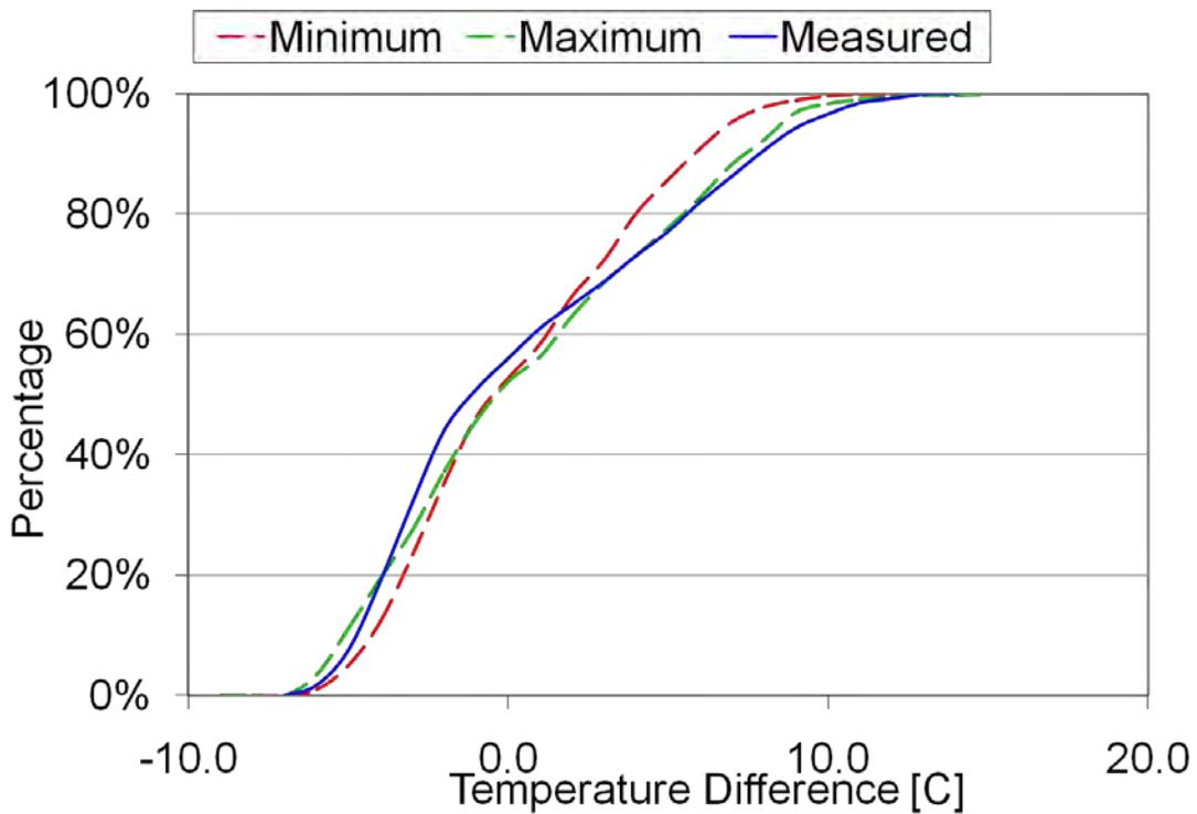
**Figure 2-28: Measured versus modeled cumulative frequency distribution for thermal gradient through JPCP pavement in March with  $k = 0.94 \text{ BTU / hr-ft-}^\circ\text{F}$ , the adjusted thermal conductivity value.**
