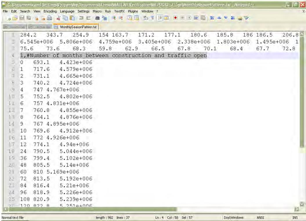
**Figure 4-4: MEPDG input file specifying number of months between construction and traffic open.**
