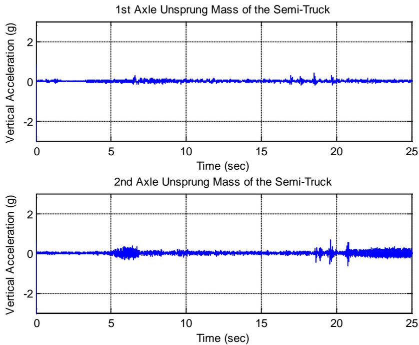
**Figure 2.10: Axle vibrations on semi-truck at 10 mph.**
