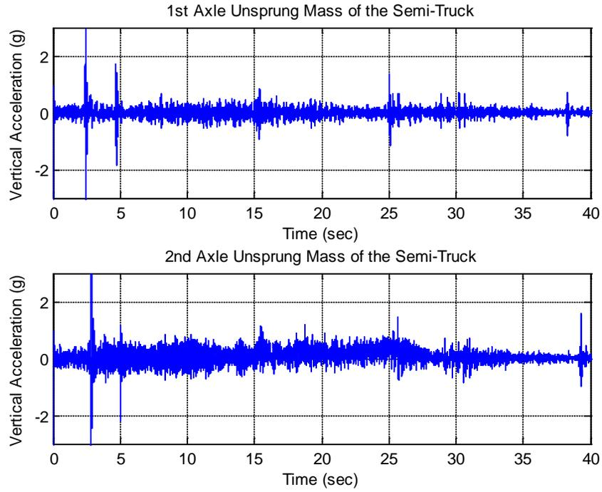
**Figure 2.13: Axle vibrations on semi-truck at 40 mph.**
