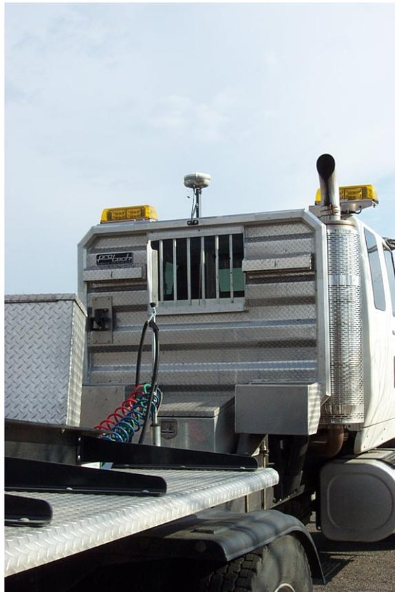
**Figure 2.17: Differential GPS system located above tractor cab.**
