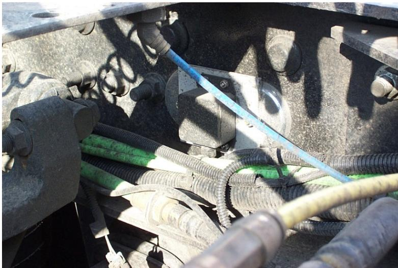
**Figure 2.5: Accelerometer at front left top of tractor.**
