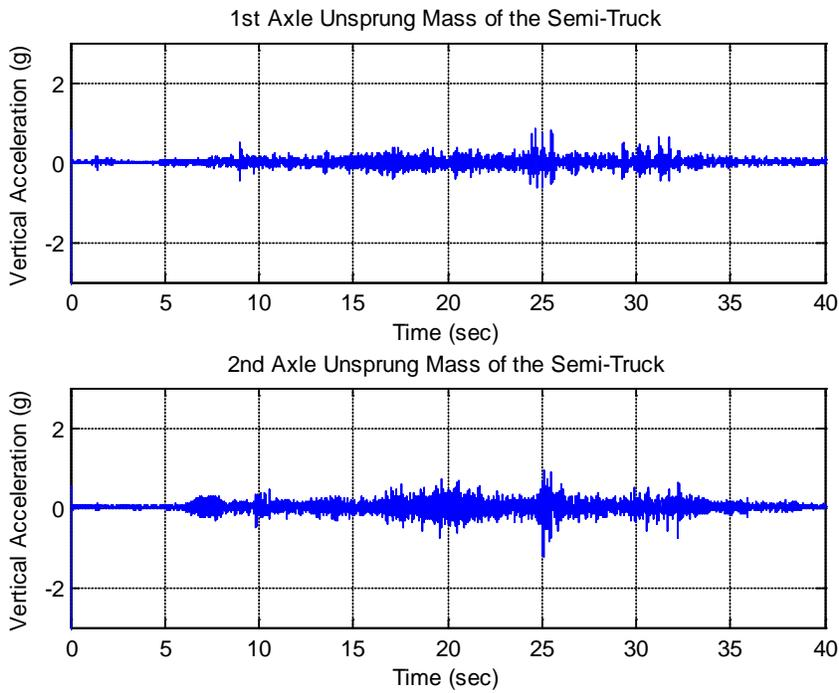
**Figure 2.12: Axle vibrations on semi-truck at 30 mph.**
