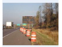
Portable changeable message signs are useful for temporary conditions, such as road construction, maintenance, work zone applications, special events and incident management.
