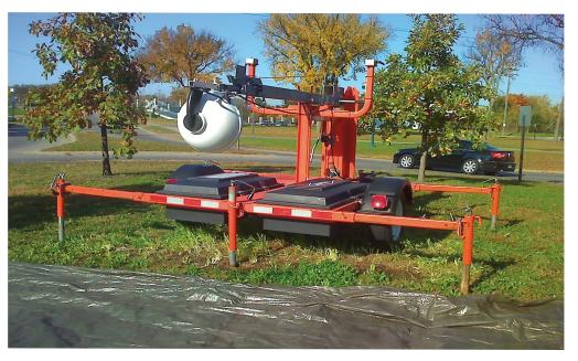
Surveillance trailers installed in the middle of roundabouts carried eight closed-circuit TV cameras and two digital video recorders to provide a clear view of the full roundabout with no blind spots.
