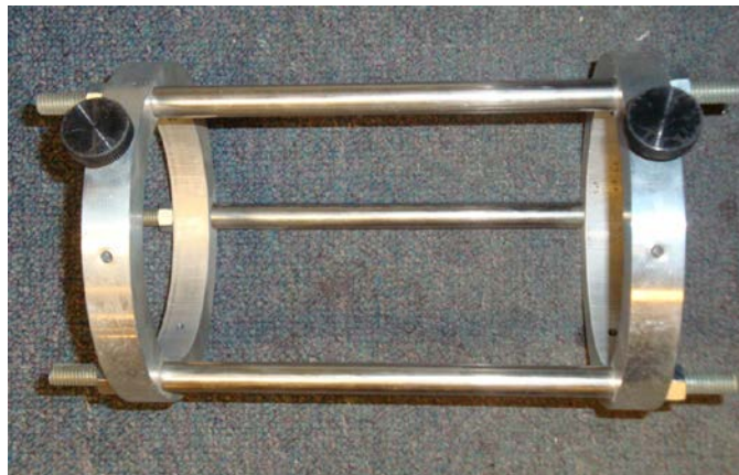
Figure 3.2: Fixture used for creating creep and shrinkage specimen molds
