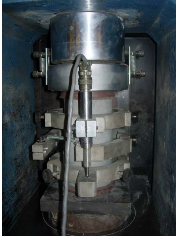
Figure 3.1: Modulus of elasticity sample in Forney concrete testing machine with compressometer attached
