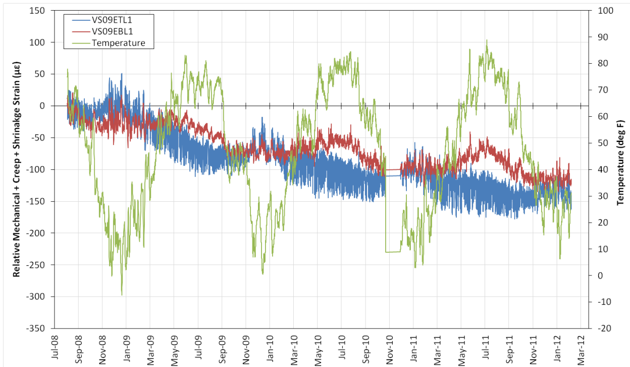
Figure 7.26: Relative mechanical strain plus creep and shrinkage strains for gages VS09ETL1 (blue; top flange at southbound Location 9) and VS09EBL1 (red; bottom flange at southbound Location 9).
