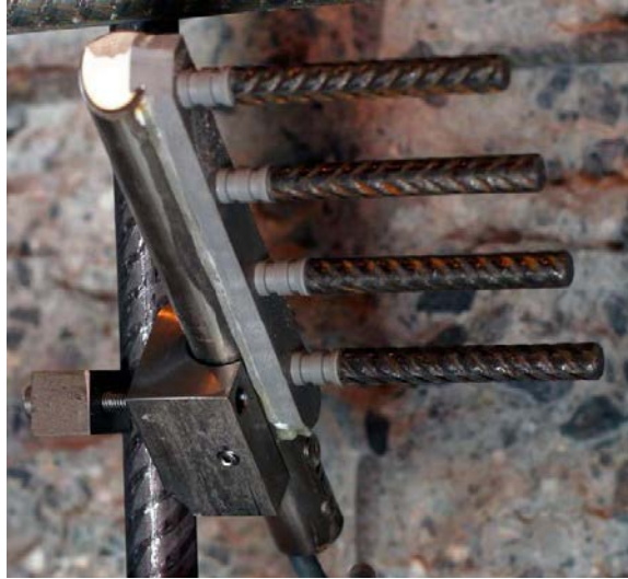
Figure 2.51: Typical Corsensys CS-040 sensor installation. Photo from Corsensys datasheet. Sensor shown is not actual sensor in bridge.
