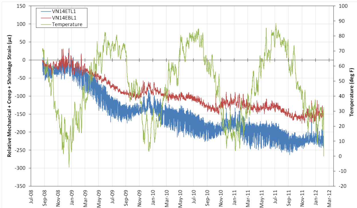
Figure 7.34: Relative mechanical strain plus creep and shrinkage strains for gages VN14ETL1 (blue; top flange at northbound Location 14) and VN14EBL1 (red; bottom flange at northbound Location 14).
