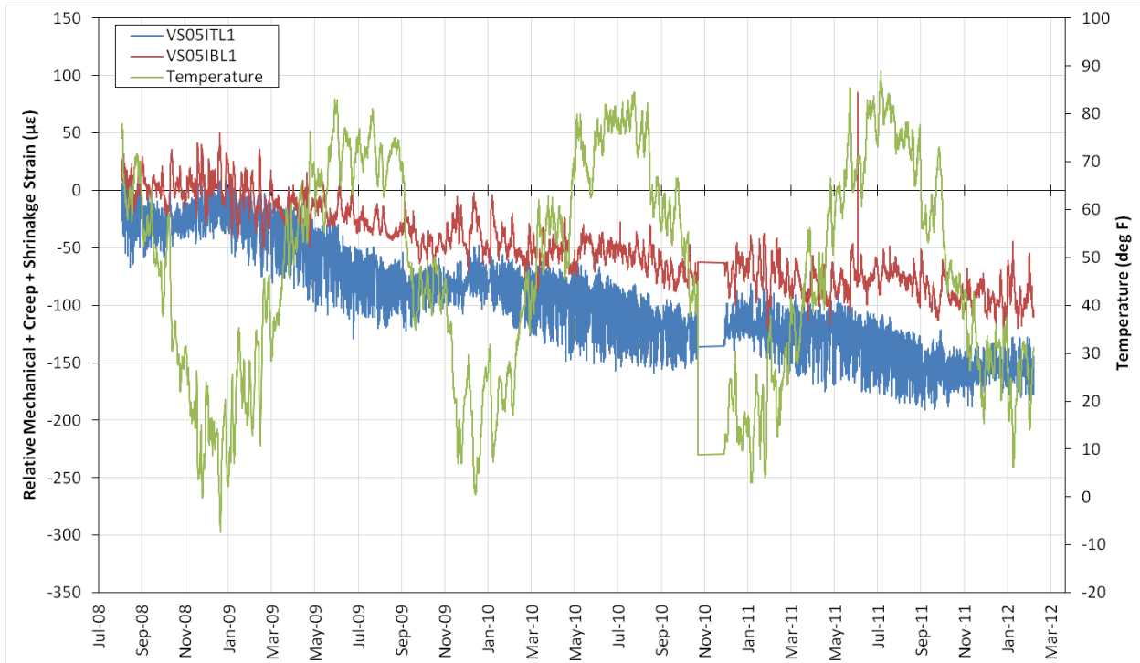
Figure 7.23: Relative mechanical strain plus creep and shrinkage strains for gages VS05ITL1 (blue; top flange at southbound Location 5) and VS05IBL1 (red; bottom flange at southbound Location 5).
