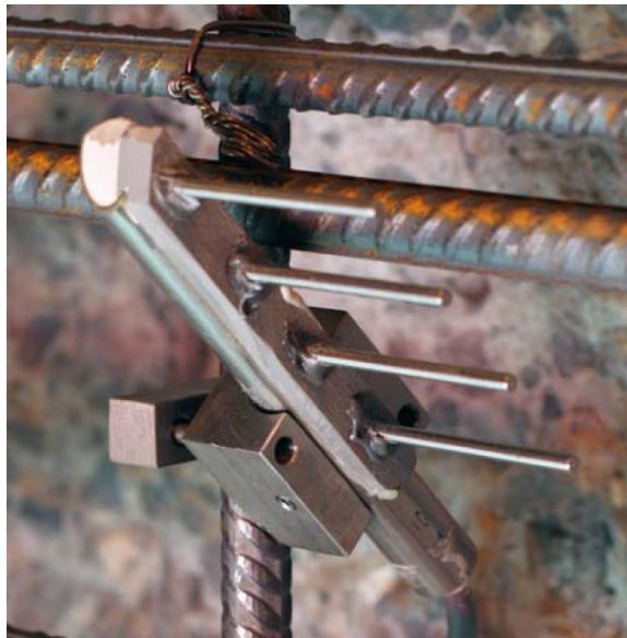
Figure 2.52: Typical Corsensys CS-402 sensor installation. Photo from Corsensys datasheet. Sensor shown is not actual sensor in bridge.
