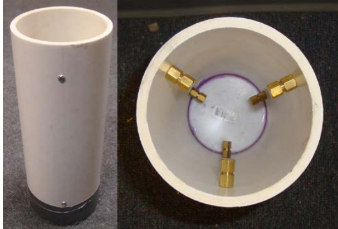
Figure 3.3: Creep and shrinkage specimen mold
