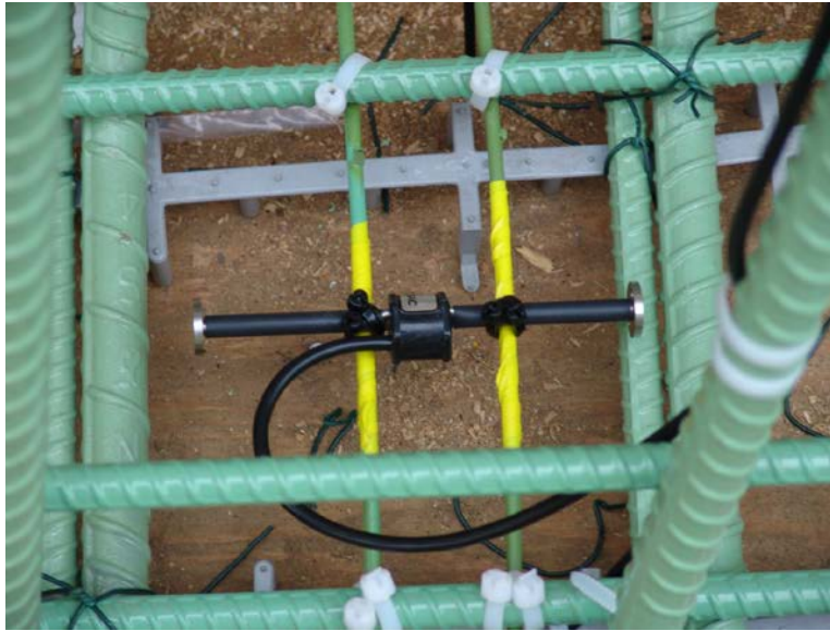
Figure 2.6: Installed Roctest EM-5 VWSG
